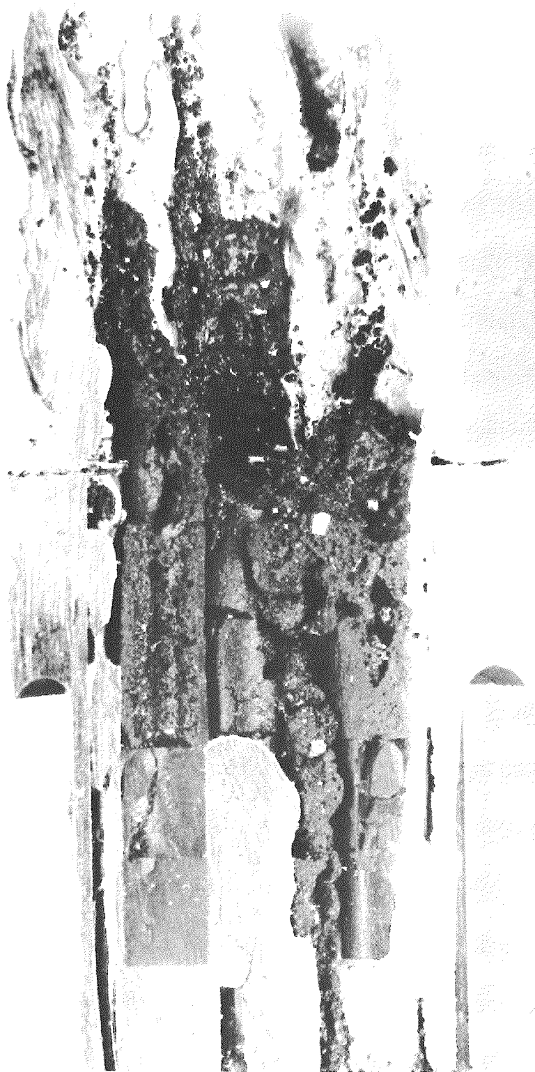
Fig. 78. Enlargement of Section A15F (see Fig. 68a) Showing Porosity around Central Void in Fuel Pellets. Mag. \sim 3.5X . Neg. No. MSD-169876.
