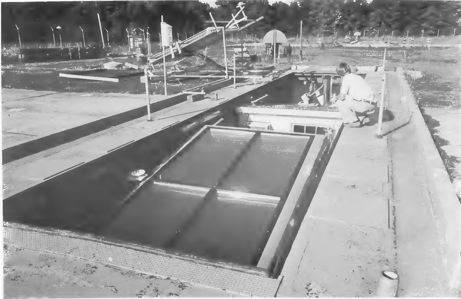
Figure 9 Solar Collector Testing Equipment Being Raised to Ground Level at the NIKI Site, NBS, Gaithersburg, Maryland.
