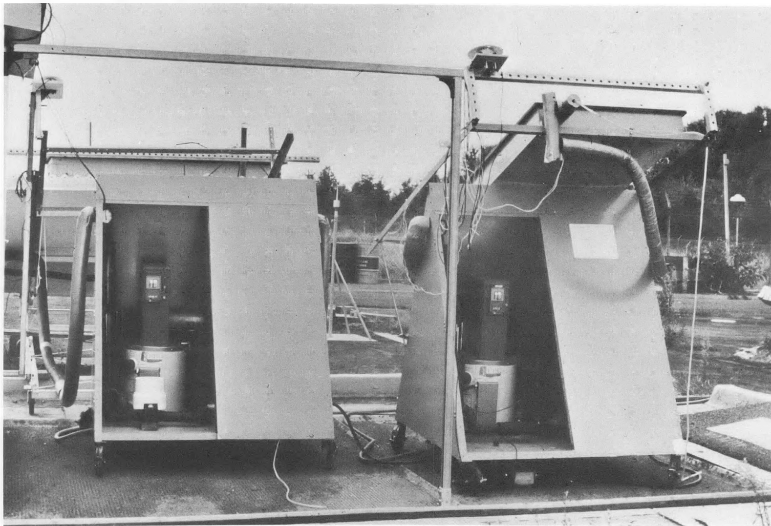
Figure 14 Test Stands for Liquid-Heating Solar Collectors as Seen from the North of the NIKI Site, NBS, Gaithersburg, Maryland.
