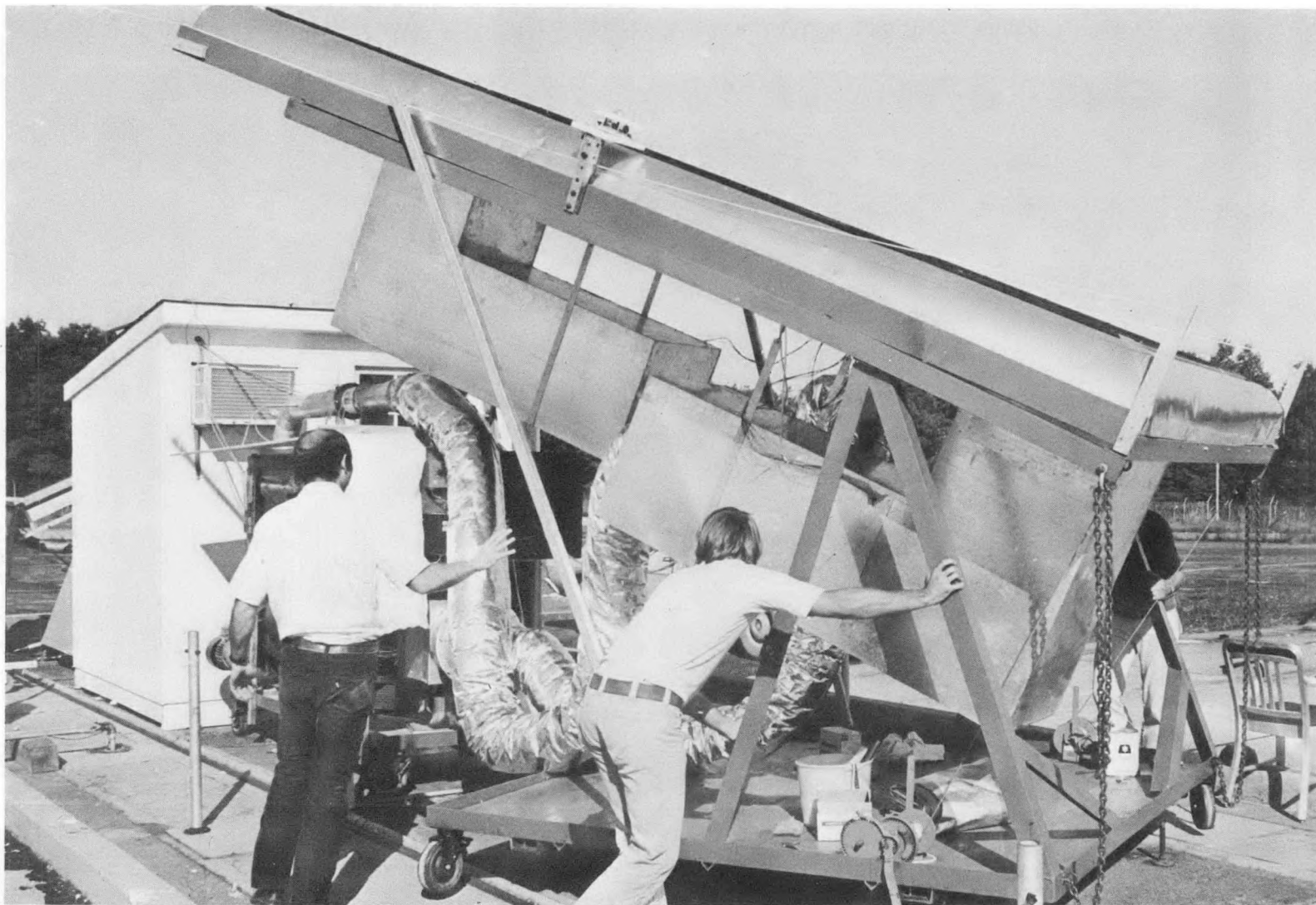
Figure 23 Test Stand for Air-Heating Solar Collectors being Turned into Position for Testing at the NIKI Site, NBS, Gaithersburg, Maryland.
