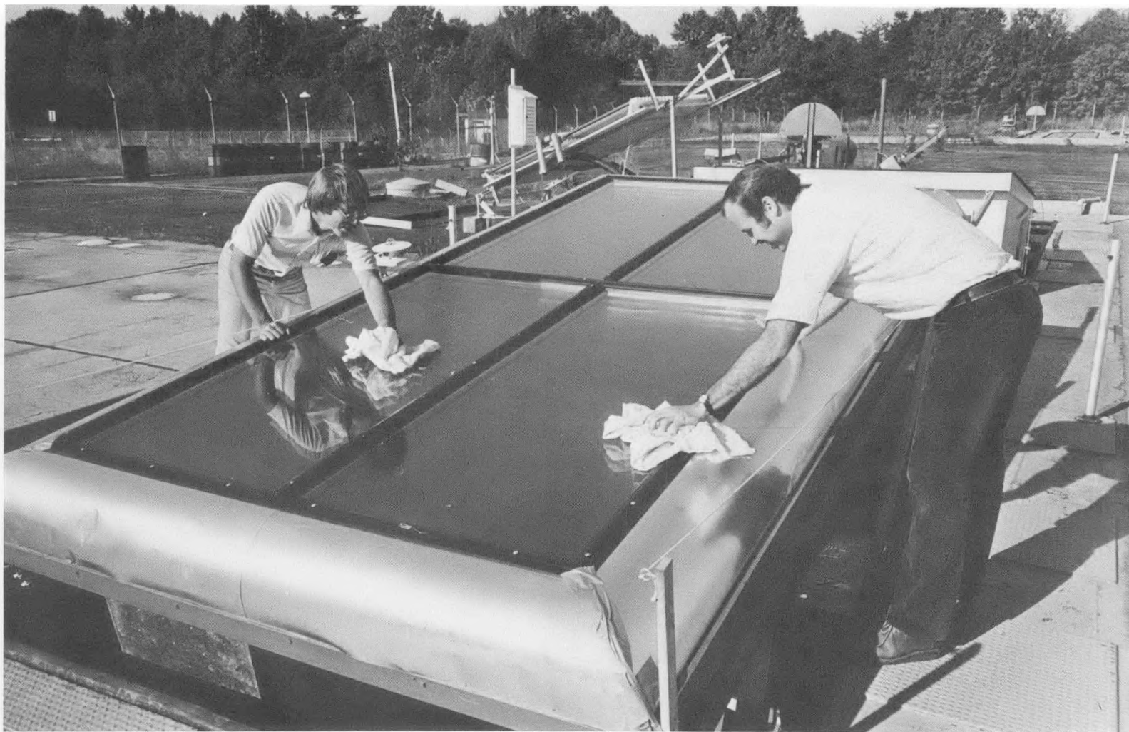
Figure 10 Air Heating Solar Collector Being Cleaned Prior to Test at the NIKI Site, NBS, Gaithersburg, Maryland.
