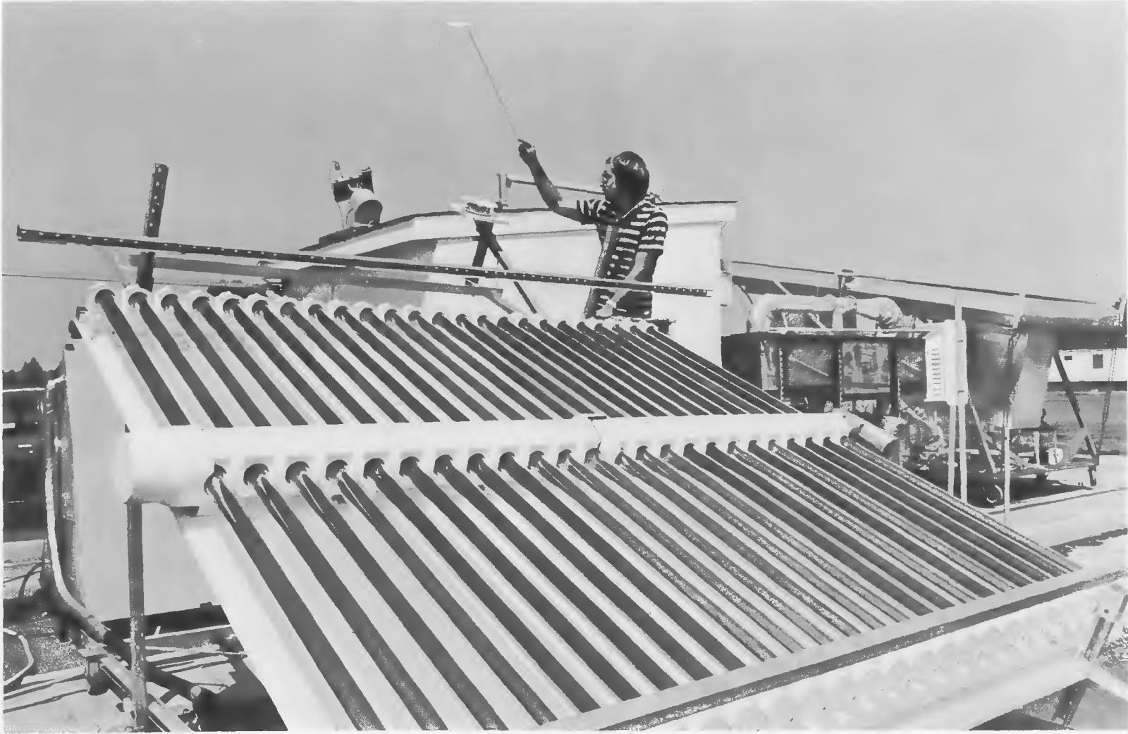
Figure 26 A Pyranometer Being Shaded During a Solar Collector Test at the NIKI Site, NBS, Gaithersburg, Maryland.
