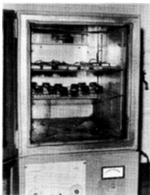
FIGURE 15.3 TEST SPECIMENS UNDERGOING EXPOSURE TO FYRQUEL GT VAPOR IN ENVIRONMENTAL CHAMBER
