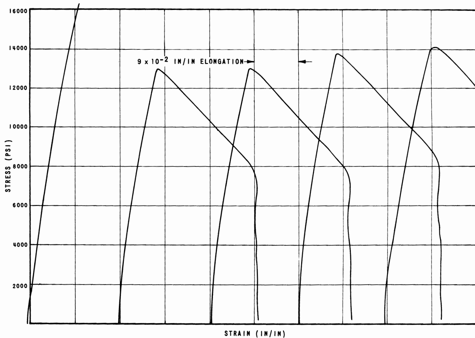
FIGURE 18.1 TENSILE STRESS-STRAIN, GLASS MAT POLYESTER LAMINATE NEMA GPO-1, AGED 135°C ONE WEEK
