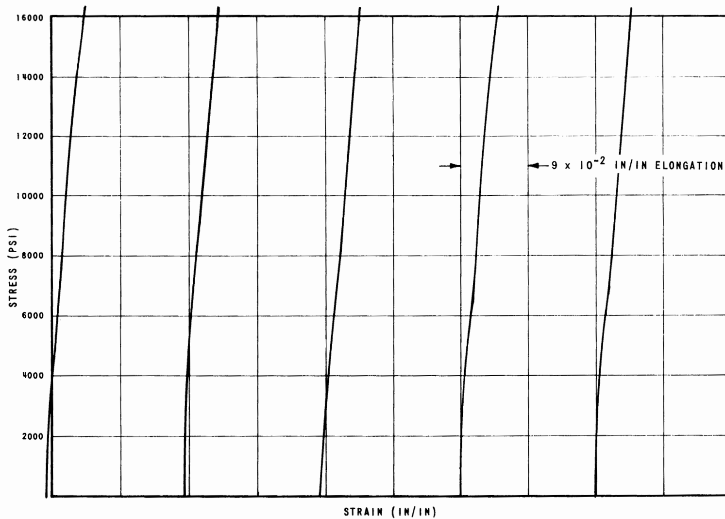
FIGURE 18.15 TENSILE STRESS-STRAIN GLASS MELAMINE LAMINATE NEMA G-9, AGED 135°C ONE WEEK
