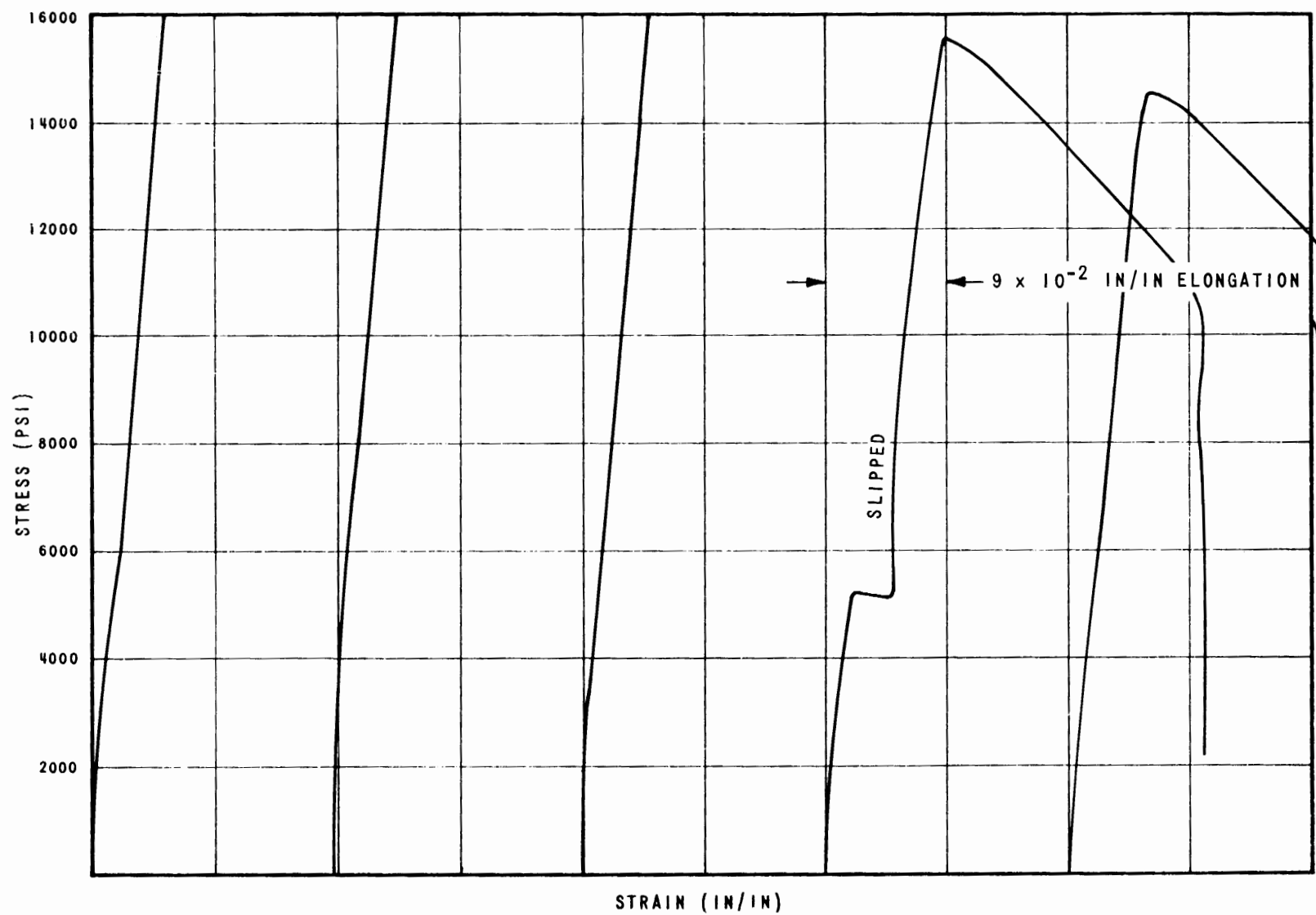
FIGURE 18.39 TENSILE STRESS-STRAIN, GLASS EPOXY LAMINATE NEMA G-11, AGED 135°C IN FYRQUEL LIQUID FOUR WEEKS
