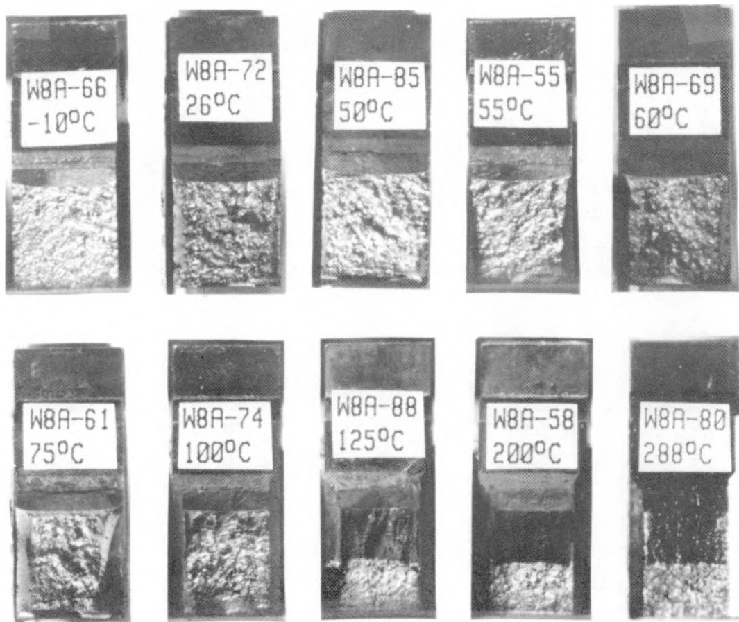
Fig. 44 Fracture surfaces for the Linde 80 weld (W8A), in the I condition to a fluence of 2.1 \times 10^{19} \text{ n/cm}^2 .
