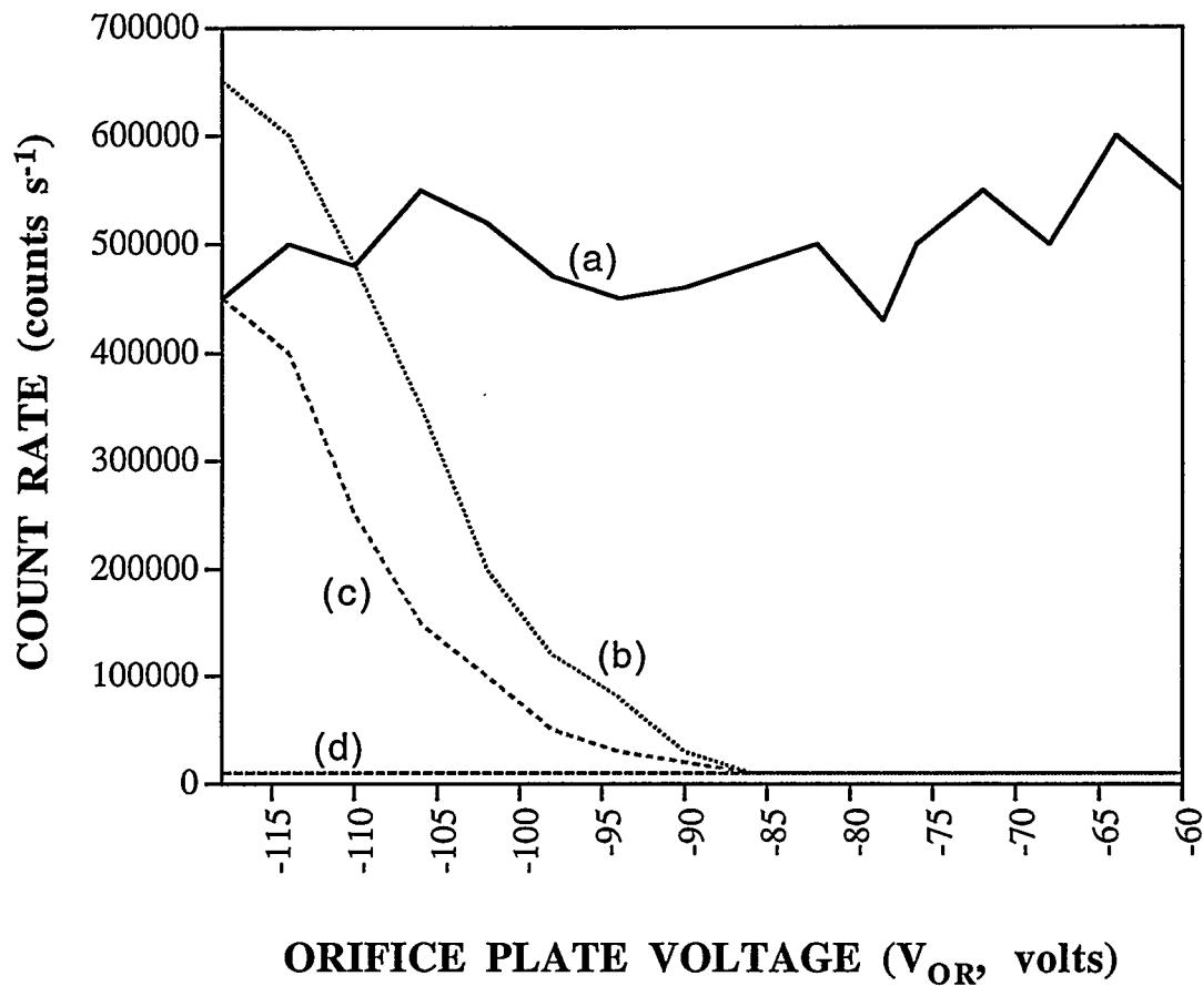
**Fig. 8** A plot of signals from the major Mn species, a)  $\text{MnO}_4^-$ ,  $m/z=119$ , b)  $\text{MnO}_3^-$ ,  $m/z=103$ , c)  $\text{MnO}_2^-$ ,  $m/z=87$ , d)  $\text{Mn}(\text{NO}_3)_3^-$ ,  $m/z=241$ , observed from a 160 ppm  $\text{KMnO}_4$  solution while varying the voltage on the orifice plate
