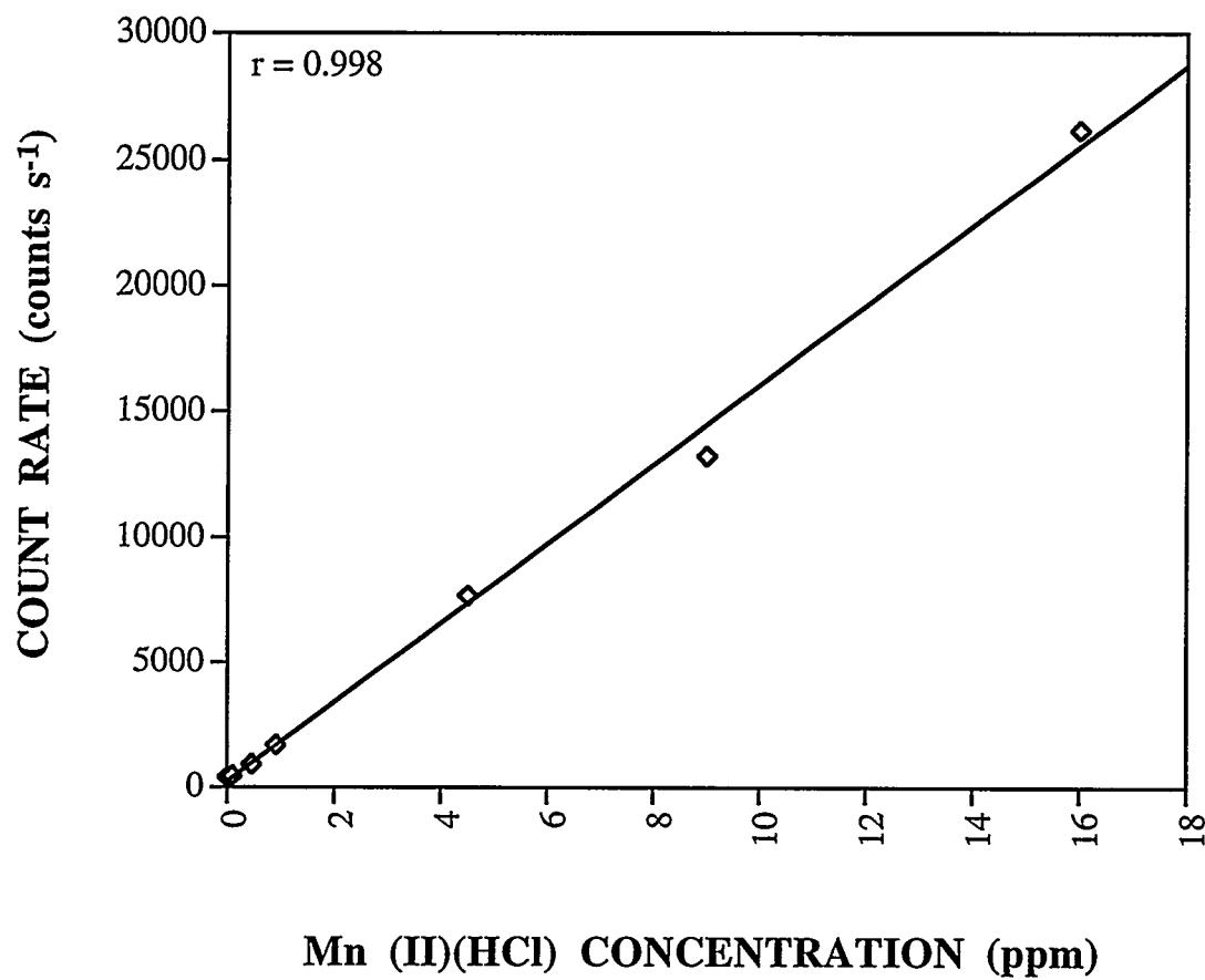
**Fig. 6** Calibration curve for Mn(II) in HCl solution
