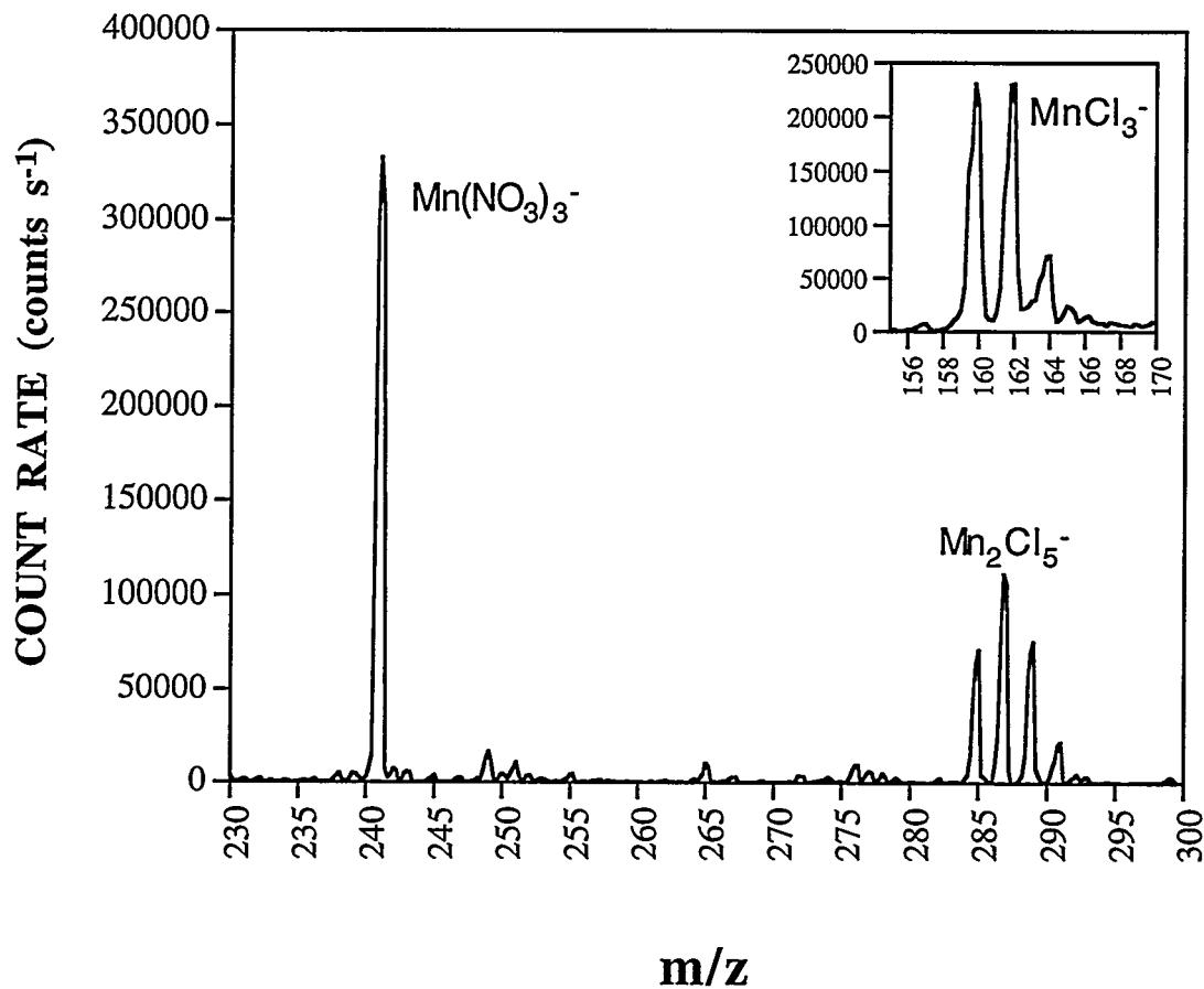
**Fig. 4** Mass spectrum of a mixture containing 10 ppm Mn(II) in  $\text{HNO}_3$  and 10 ppm Mn(II) in  $\text{HCl}$ . The inset is the region from 155 to 170 m/z
