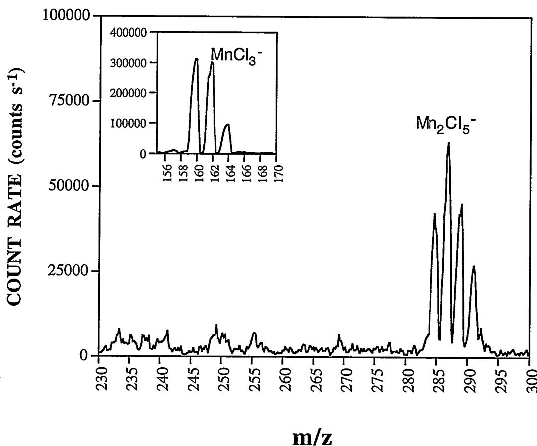
**Fig. 3** Mass spectrum of a 10 ppm Mn(II) in HCl solution. The inset is the region from 155 to 170 m/z
