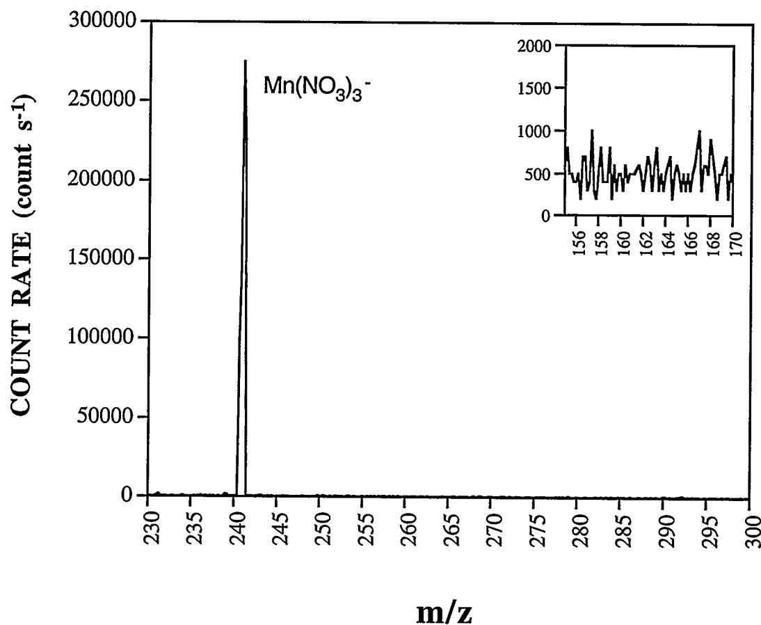
**Fig. 1** Mass spectrum of a 10 ppm Mn(II) in HNO<sub>3</sub> solution. The inset is the region from 155 to 170 m/z
