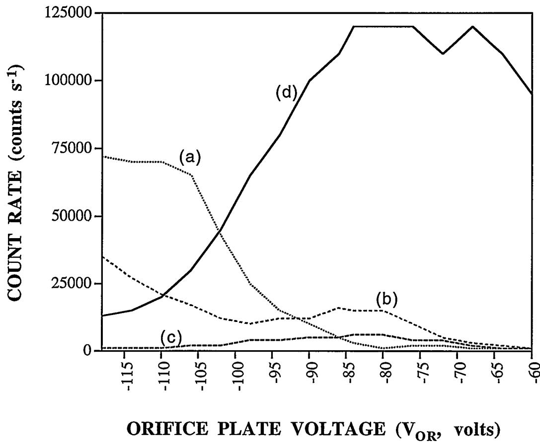
**Fig. 9** A plot of signals from the major Mn species, a)  $\text{MnO}_4^-$ ,  $m/z=119$ , b)  $\text{MnO}_3^-$ ,  $m/z=103$ , c)  $\text{MnO}_2^-$ ,  $m/z=87$ , d)  $\text{Mn}(\text{NO}_3)_3^-$ ,  $m/z=241$ , observed from a 25 ppm Mn(II) in  $\text{HNO}_3$  solution while varying the voltage on the orifice plate
