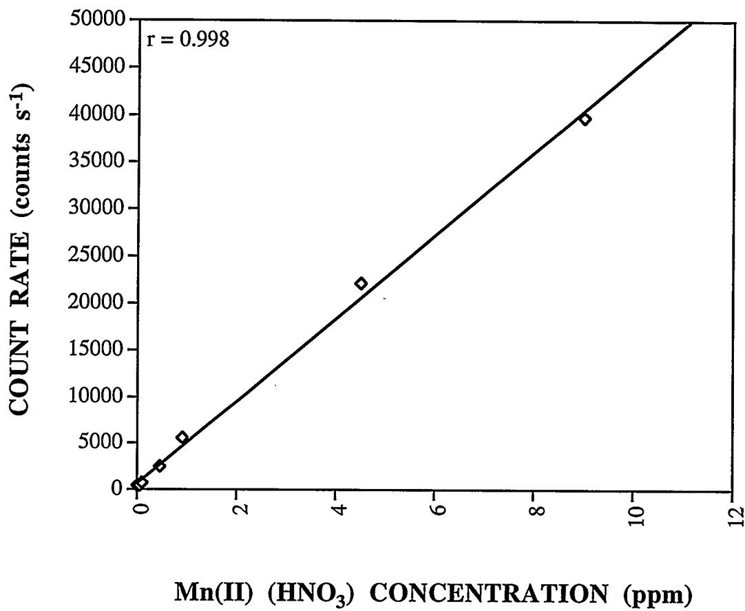
**Fig. 5** Calibration curve for Mn(II) in HNO<sub>3</sub> solution
