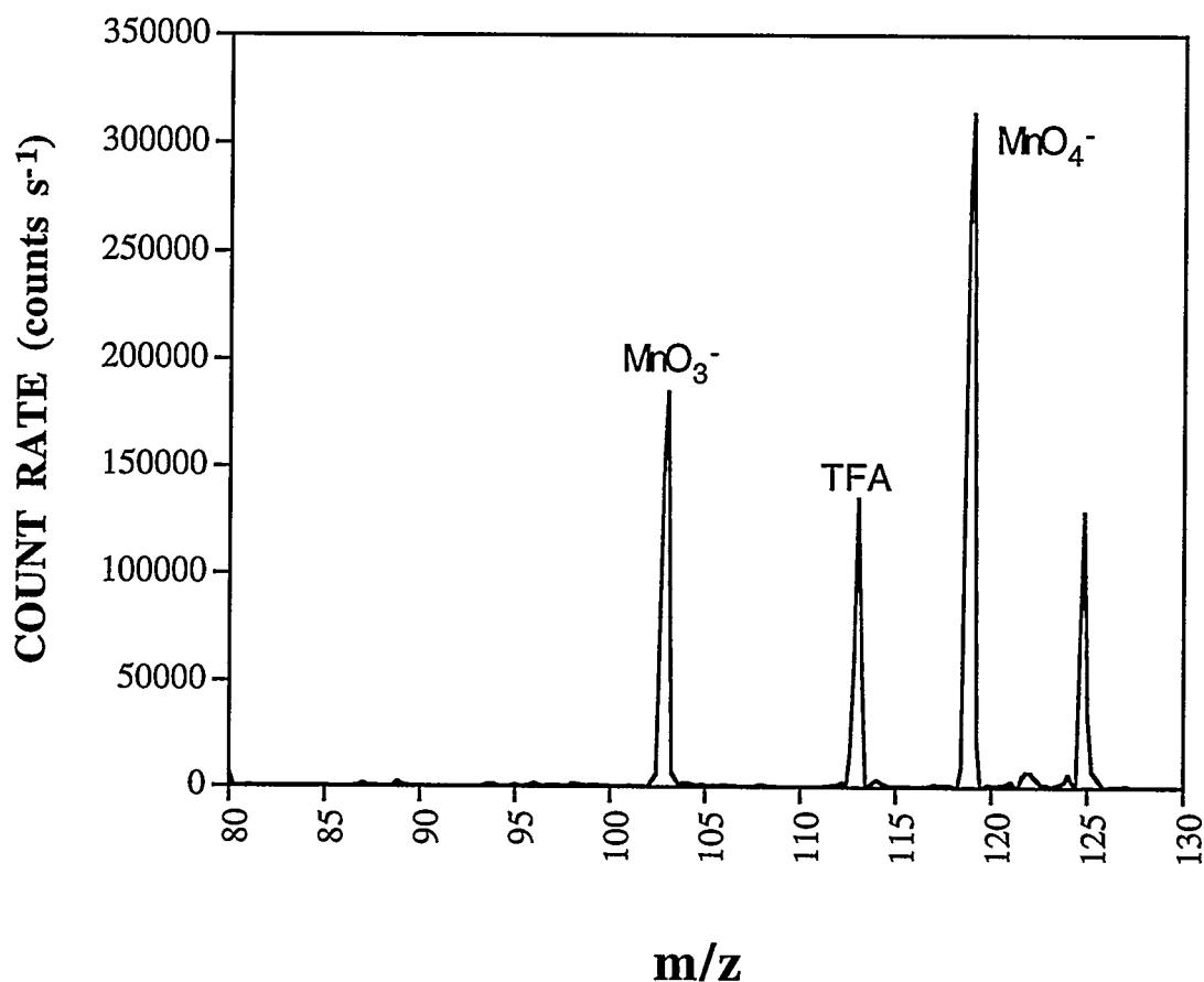
**Fig. 2** Mass spectrum of a 25 ppm Mn(II) in  $HNO_3$  solution
