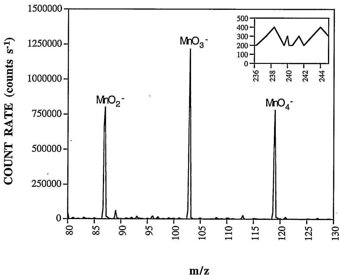
**Fig. 7** Mass spectrum of a 160 ppm  $\text{KMnO}_4$  solution. The inset is the region from 236 to 245 m/z
