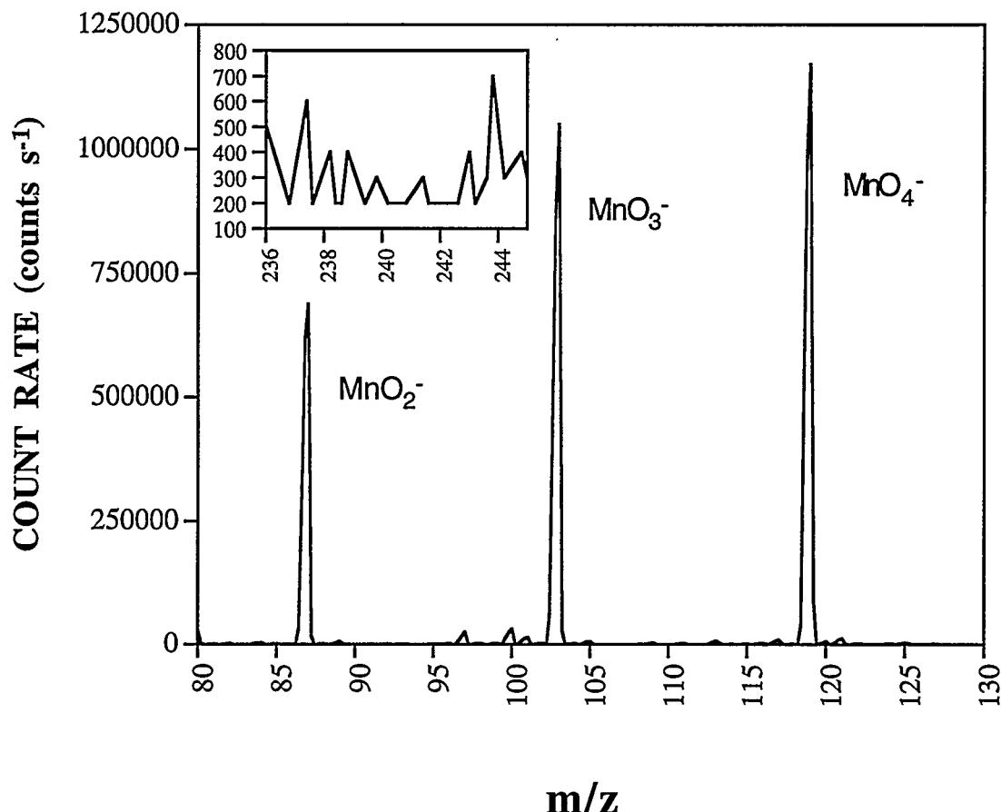
**Fig. 10** Mass spectrum of a mixture containing 160 ppm KMnO<sub>4</sub> and 25 ppm Mn(II) in HNO<sub>3</sub> solution. The inset is the region from 236 to 245 m/z
