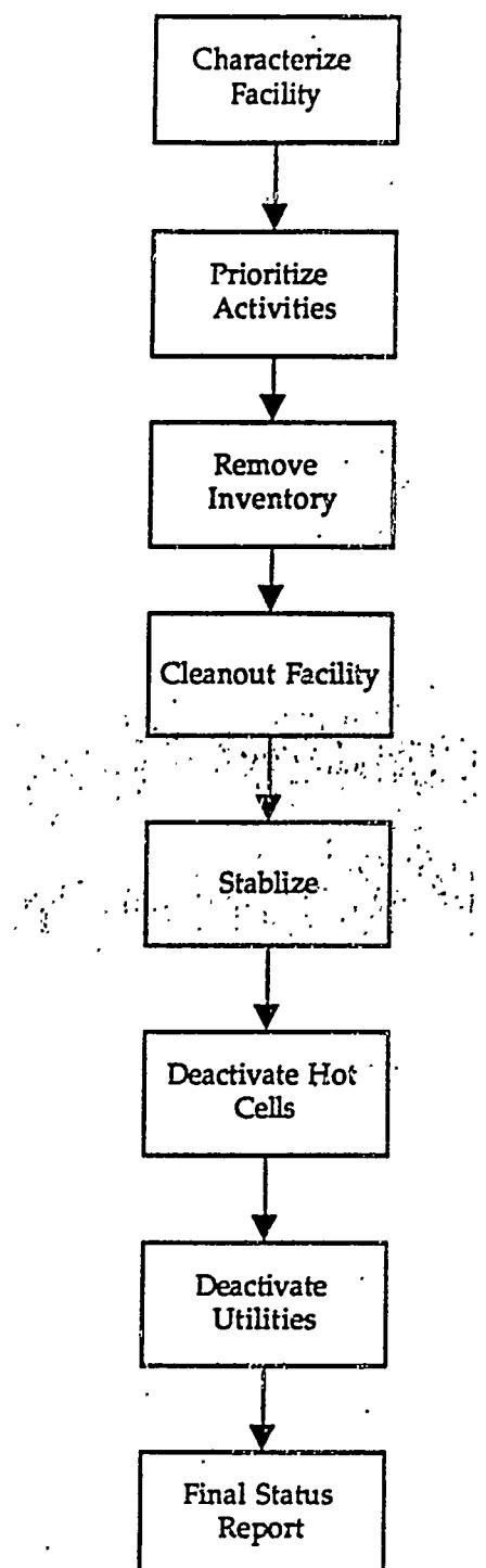
Fig. 1. Deactivation process for surplus facilities.
