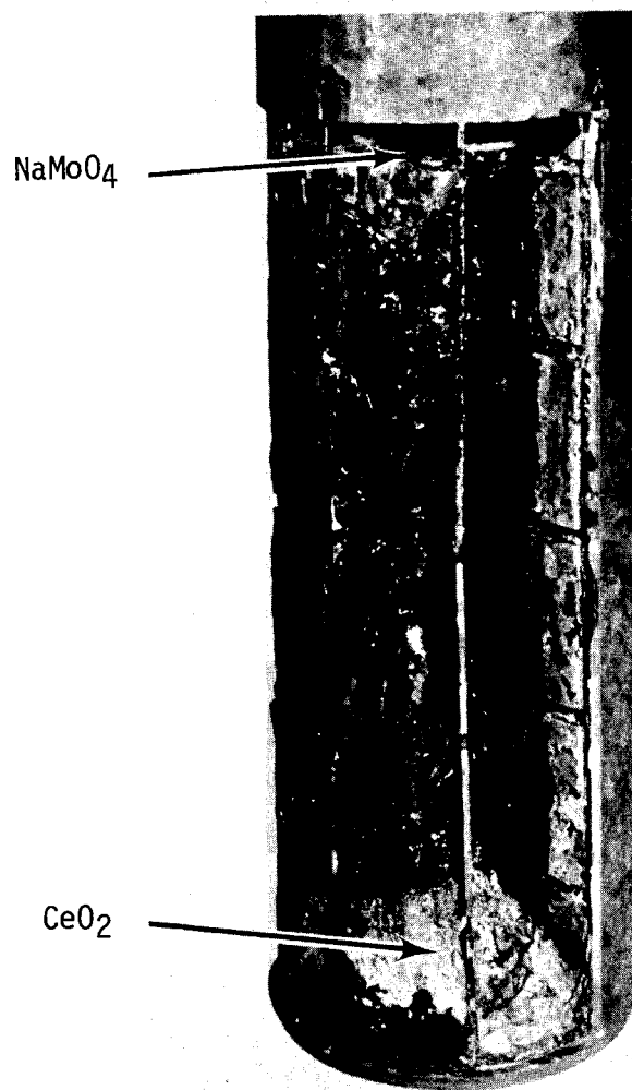
EARLY MELT SHOWING PHASE SEPARATIONS
