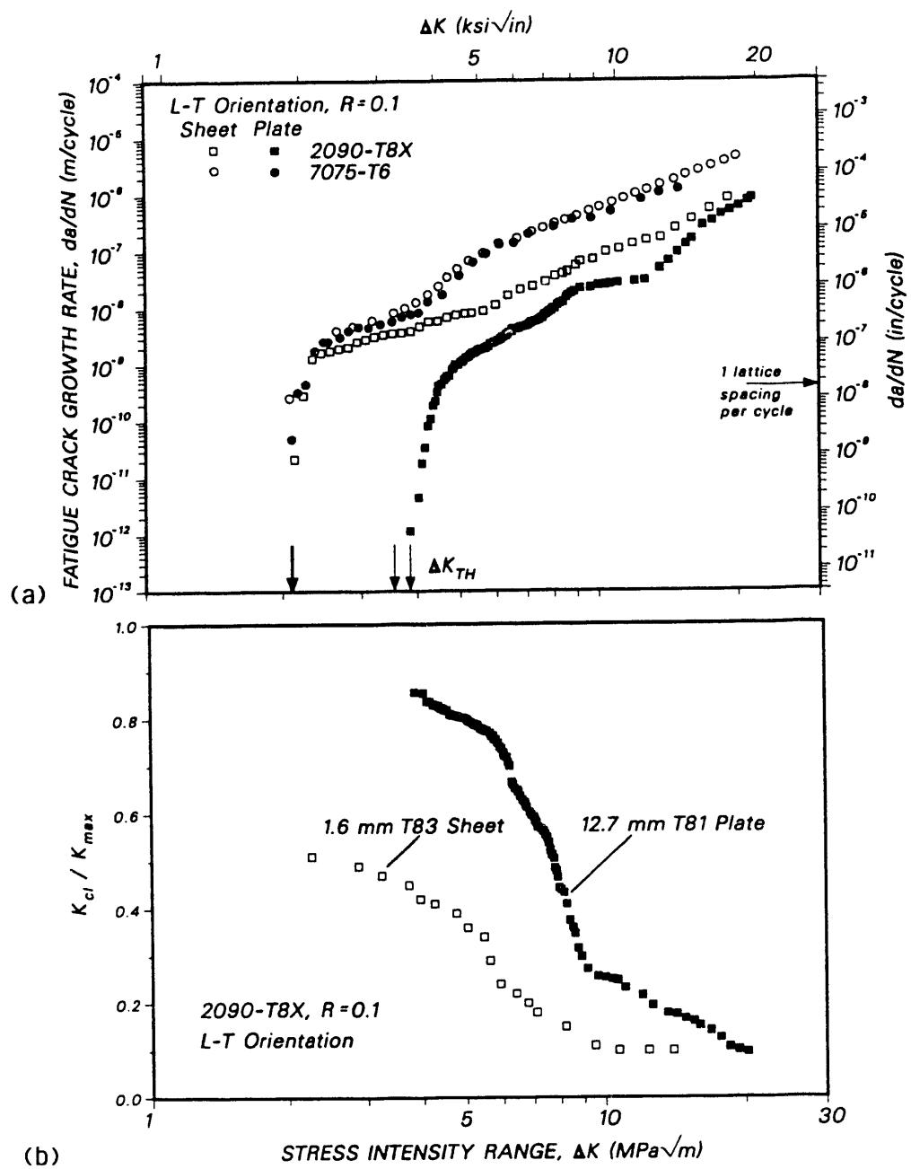
Figure 2. a) Fatigue-crack growth and b) crack-closure ( $K_{cl}/K_{max}$ ) behavior in 2090-T8 sheet and plate at  $R = 0.1$ , as a function of the nominal stress-intensity range  $\Delta K$ . Growth-rate data are compared with corresponding results on 7075-T6 (7,14). T81 plate data obtained on 6.4 mm thick specimens (T/2 location).
