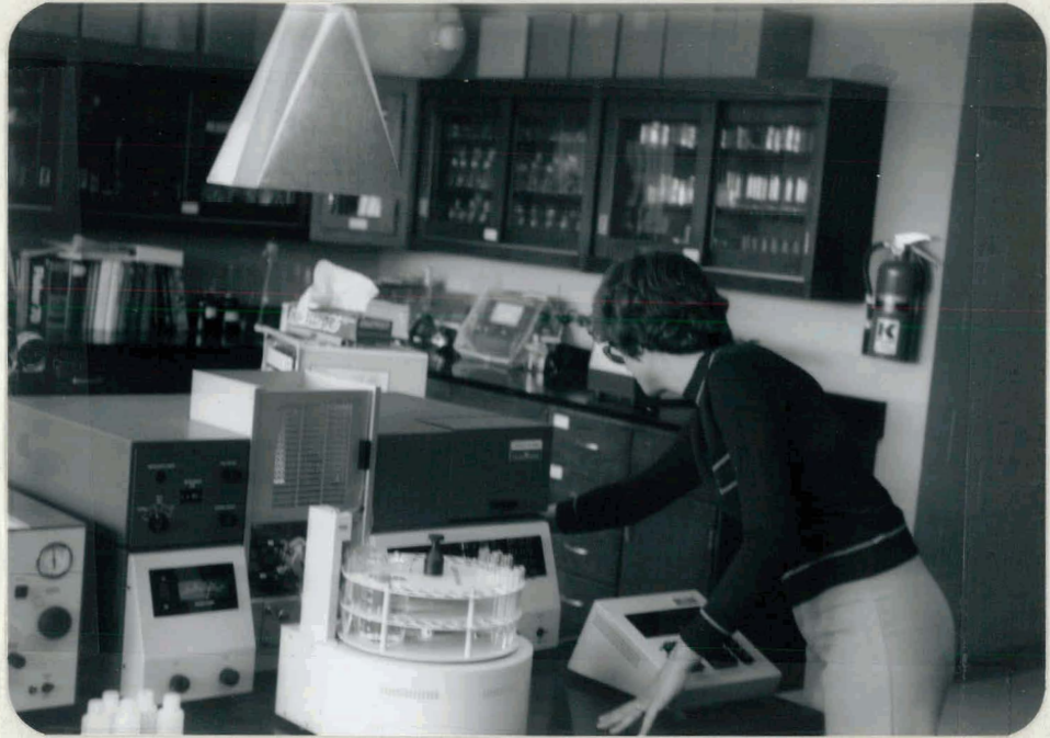
Fig. 9. Soil and plant analysis for nutrients with atomic absorption unit.
