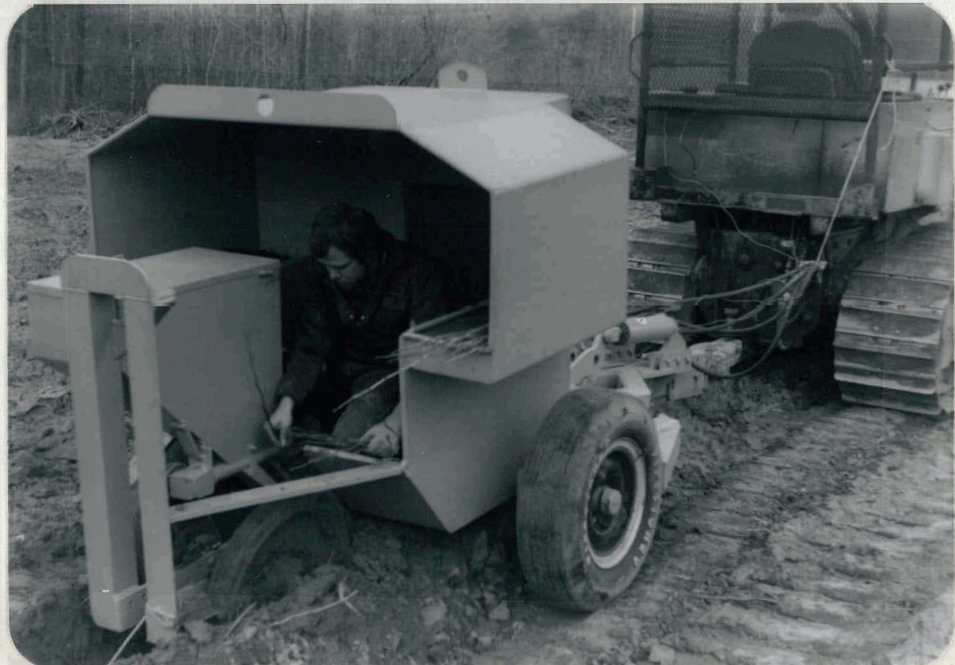
Fig. 8. One objective of the SRP planting was to test the feasibility of applying fertilizer in the planting silt. Custom-built fertilizer hopper at the right of the man planting the seedling.
