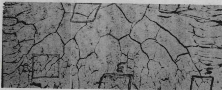
FIGURE 19. Effect of Interaction of Hot-Press Pressure and Pressure Ramp on Microstructure of MHW Pellets. a. High Hot-Press Pressure, Fast Ramp.
