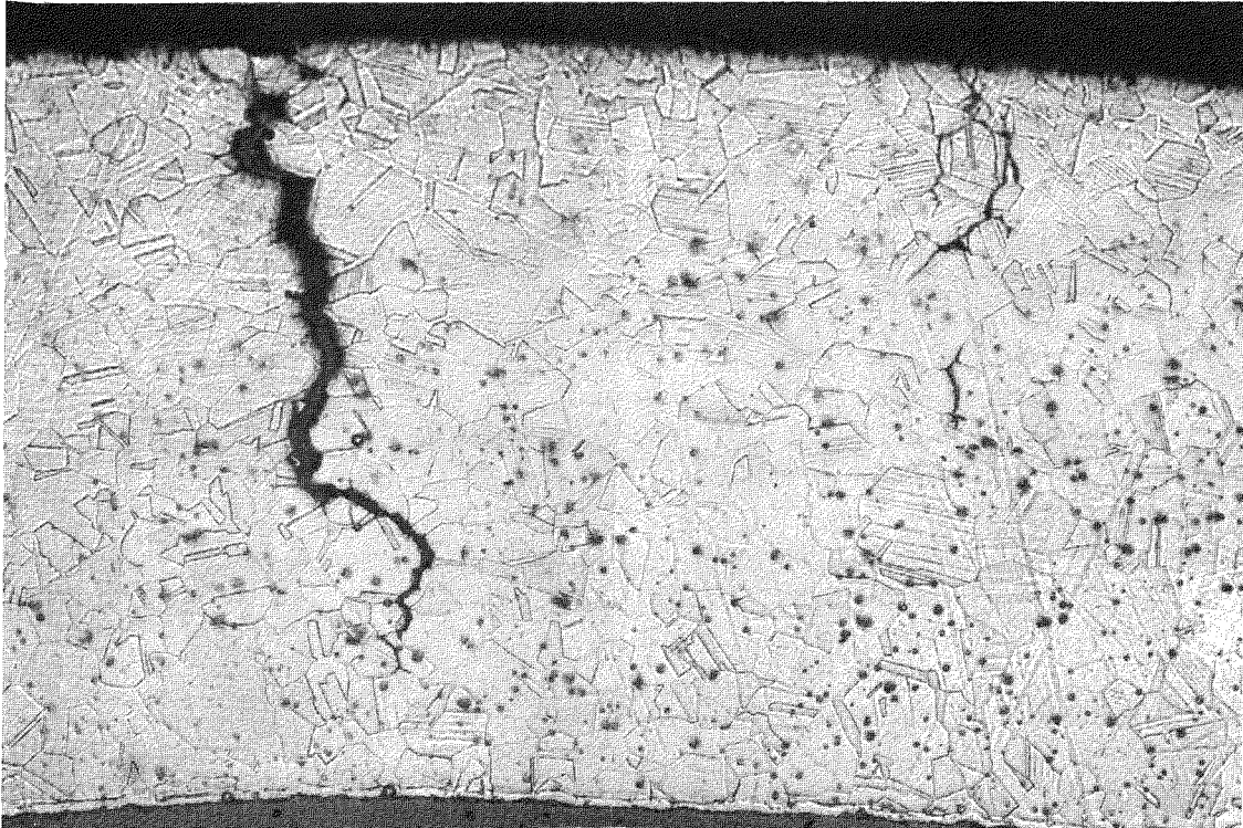
FIGURE 19. Appearance Of The Two Cracks In Rod 157E01 At 64 Inches In Etched Condition (Etchant — Glyceregia)
