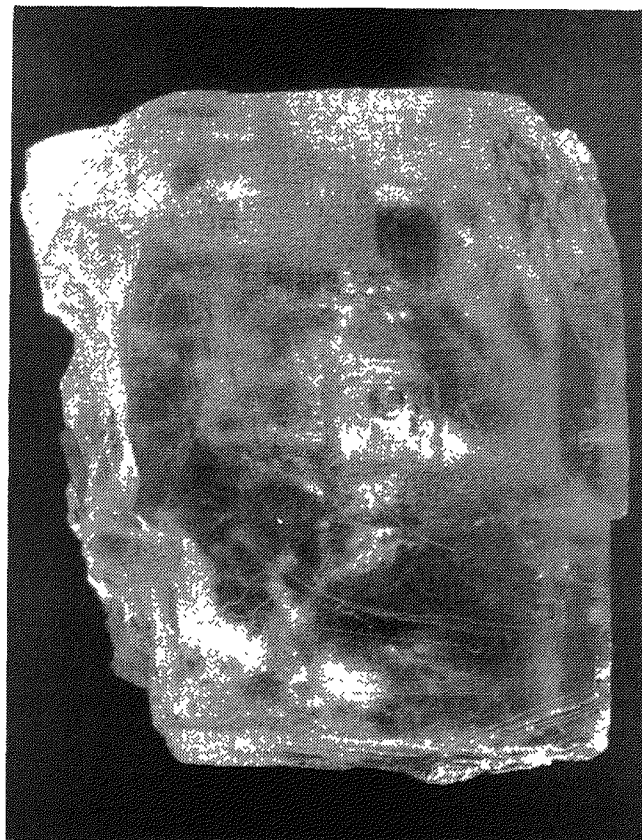
Figure 5. Sample of Lower Salado Formation Salt From the Level of the Facility Horizon at 2150 ft. (This example contains extremely large fluid inclusions in clear, recrystallized salt, such as that seen in the center of the photograph (with bubble). In the unrecrystallized upper left corner, the milky bands composed of thousands of microscopic fluid inclusions define a primary "hopper" crystal. Scale bar = 0.5 cm.)
