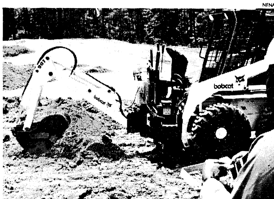
Figure 9. Remote Control of BOBCAT with Backhoe Attachment
