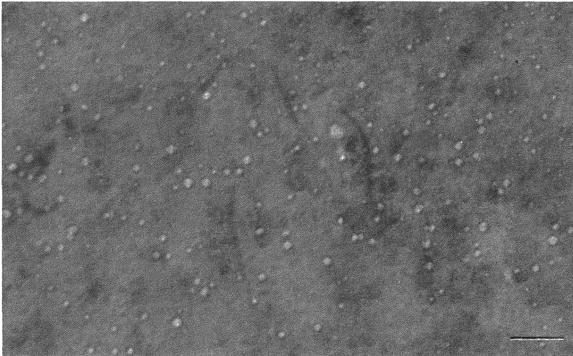
Figure 4.4. TEM micrograph showing the crystallographic shape of cavities found in the damage profile for iron. Scale marker is 100 nm.
