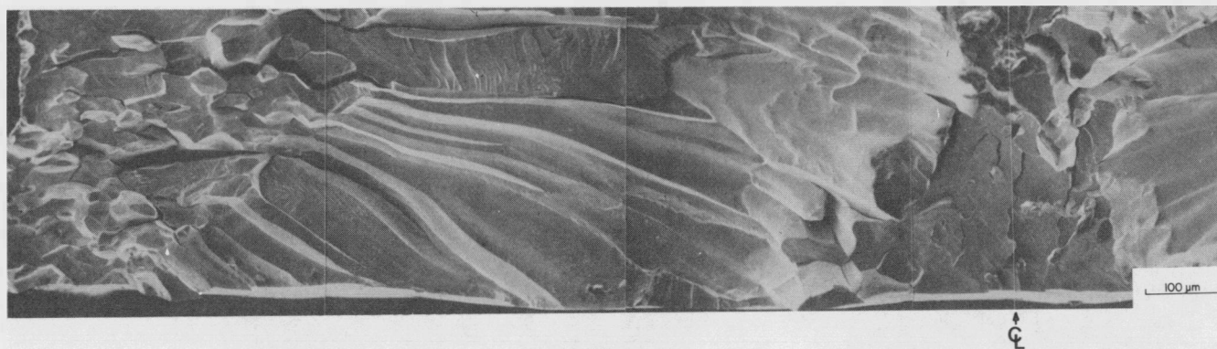
Fig. 12. Scanning electron microscopic fractograph of the DOP-26 specimen with a narrow longitudinal weld impact-fractured at 900°C and 61 m/s; postweld heat treatment: 1 h at 1500°C.
