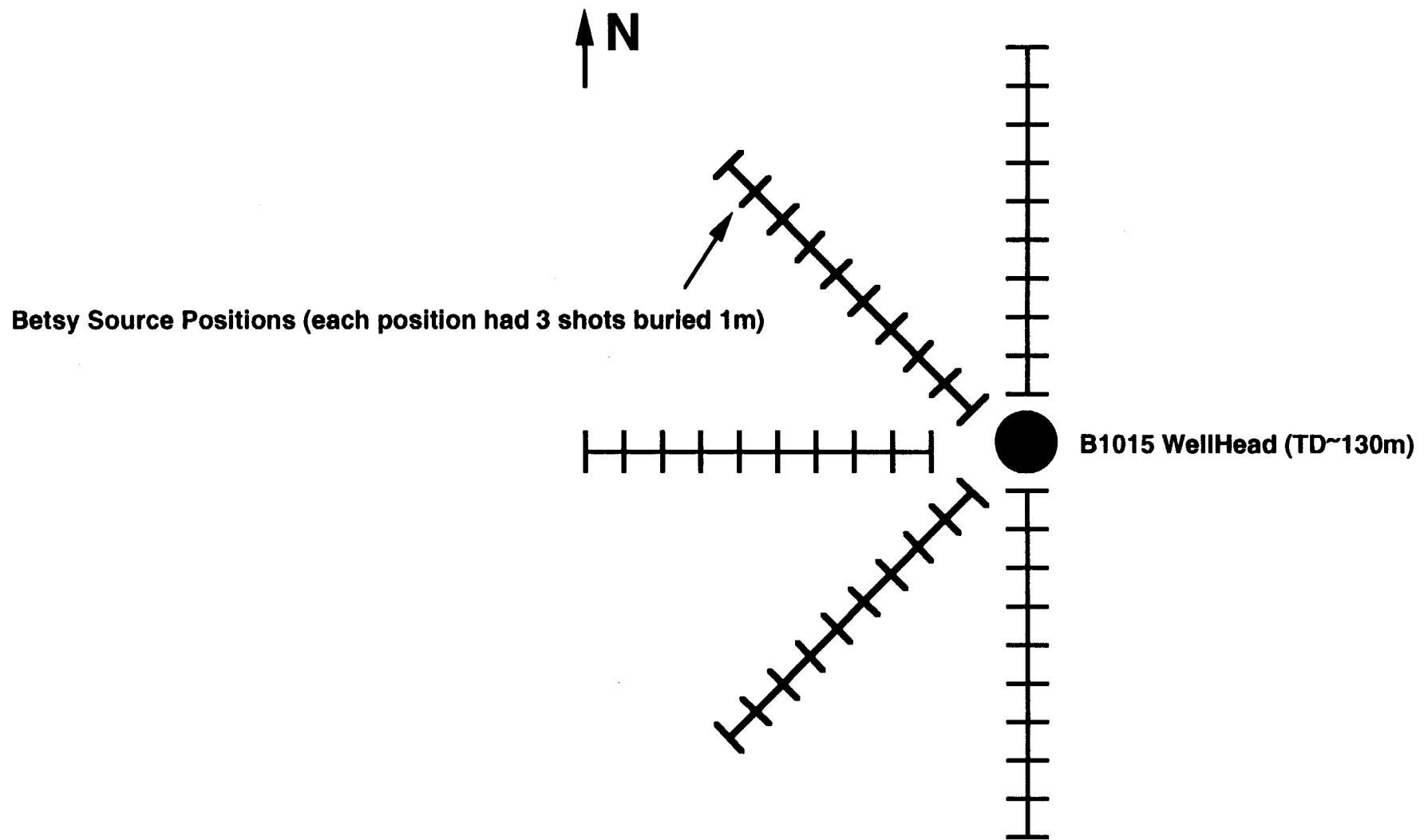
**Figure 5.** Map view of offset VSP acquisition geometry.
