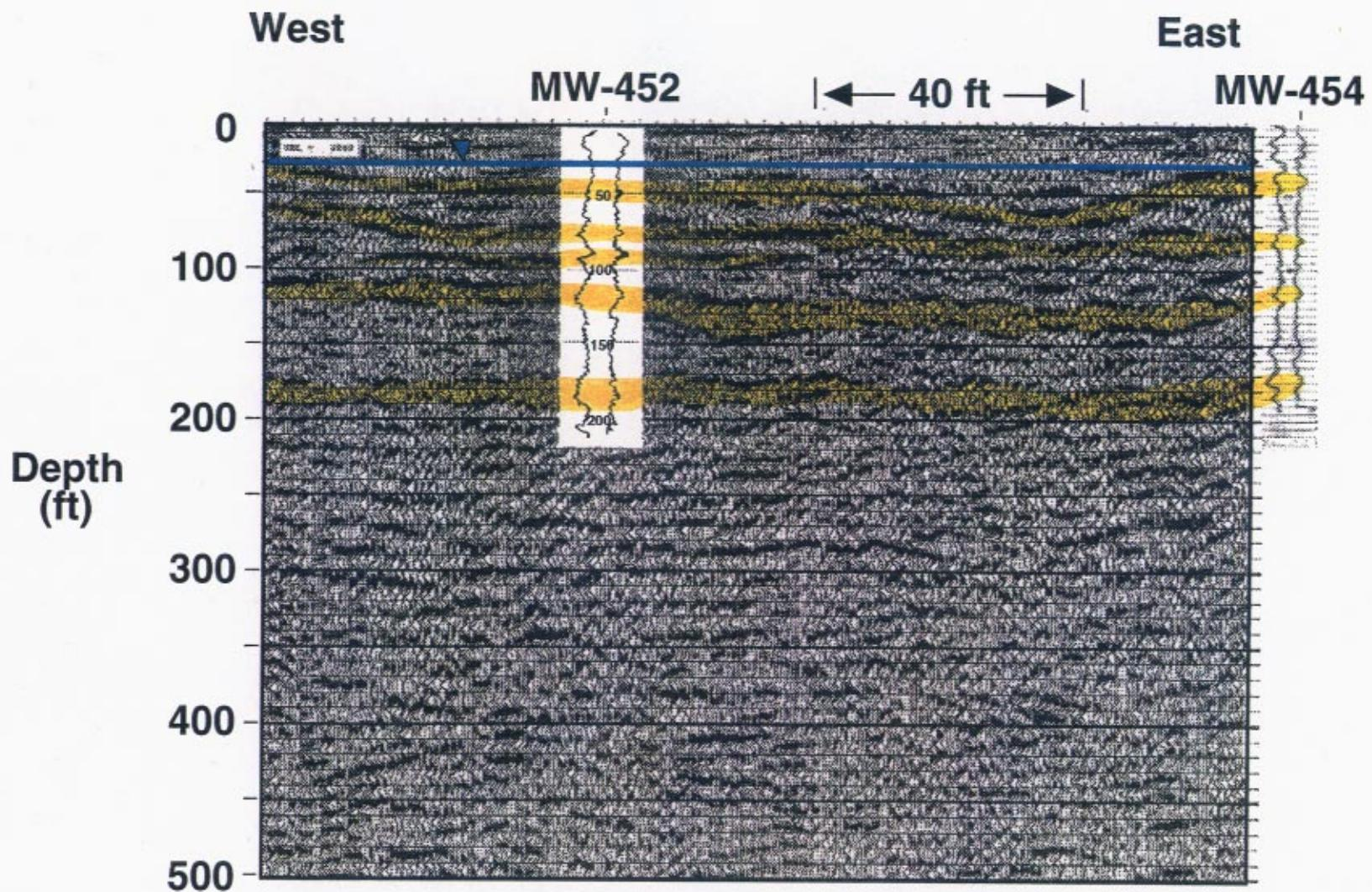
Figure 1. Brute stack of 2-D reflection line.
