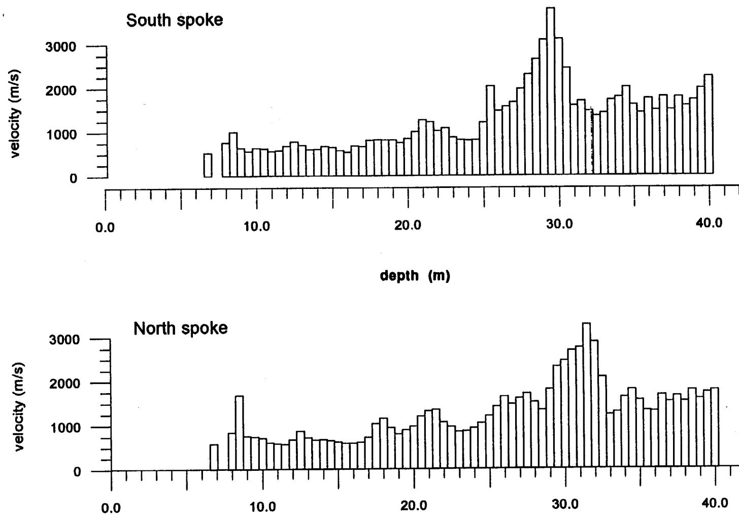
Figure 4. Well B-1015 Interval velocities.
