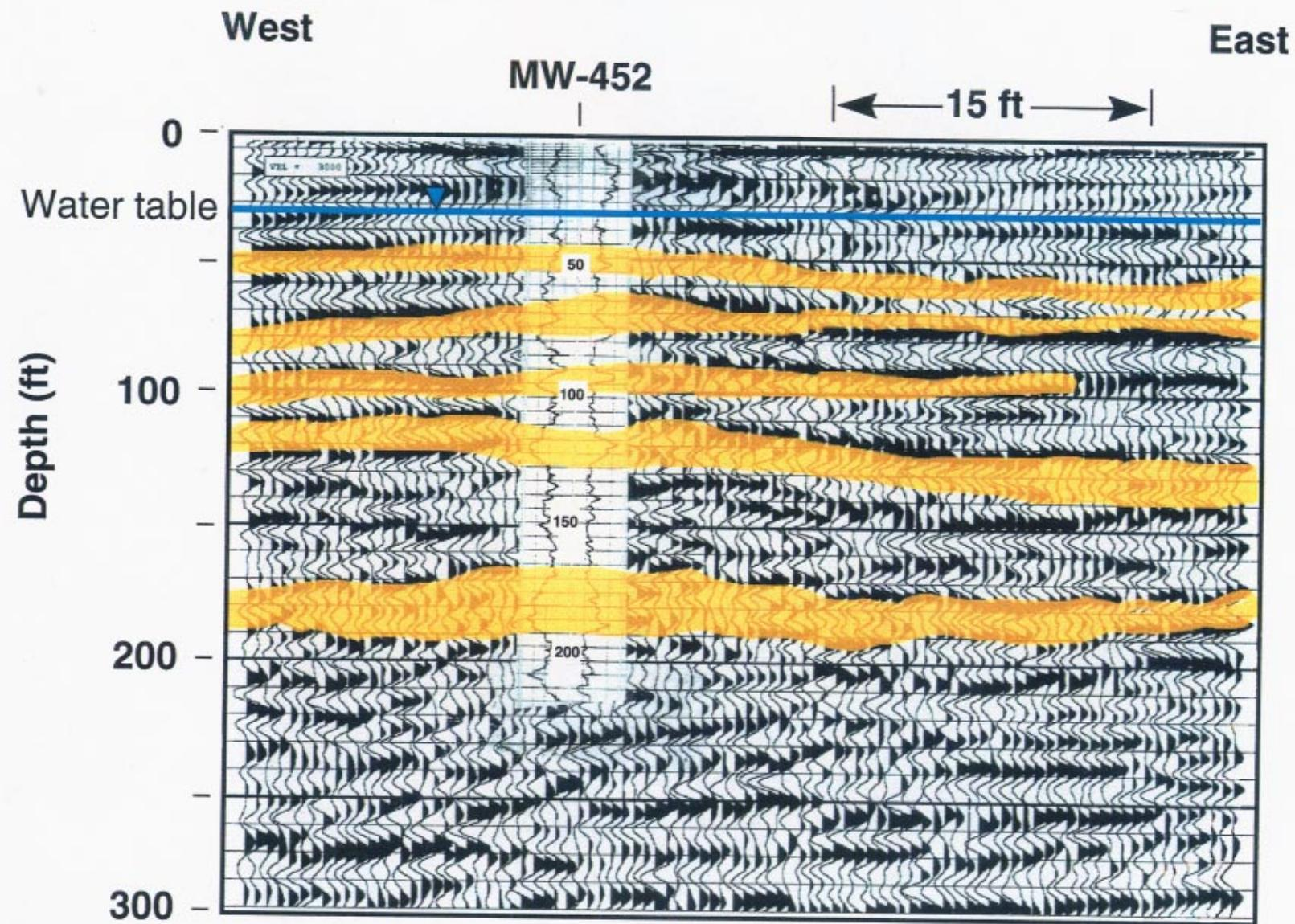
Figure 2. 2-D reflection line after extensive processing.
