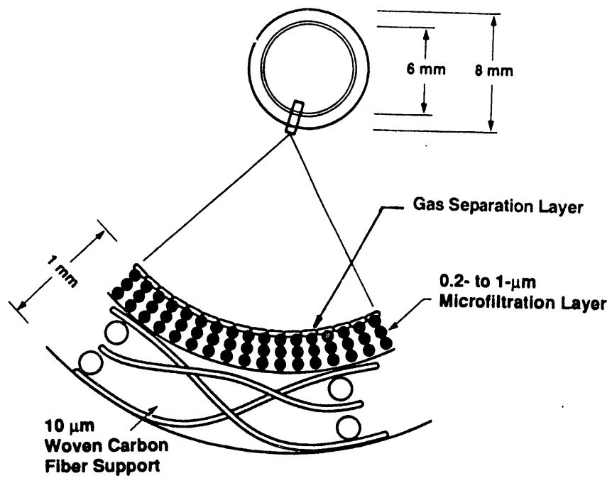
**Figure 3-1. Schematic of carbon composite membrane structure.**
