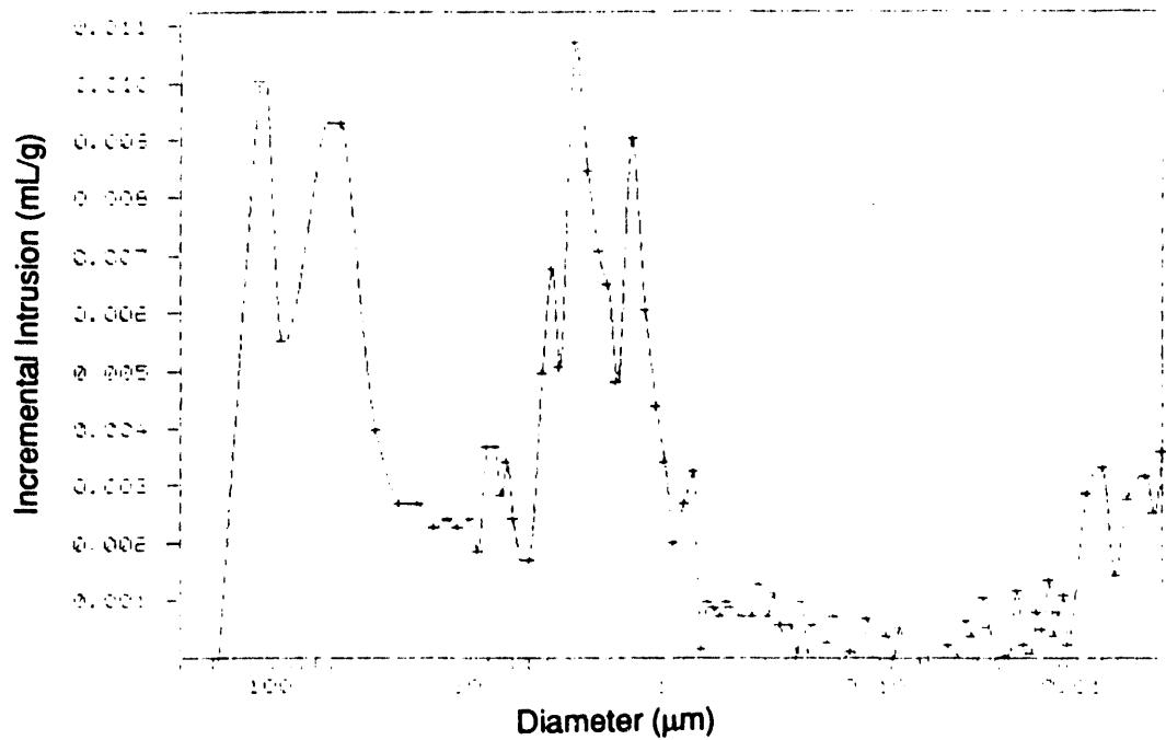
**Figure 3-3.** Pore size distribution for a 0.2- $\mu\text{m}$  unmodified carbon membrane sample.
