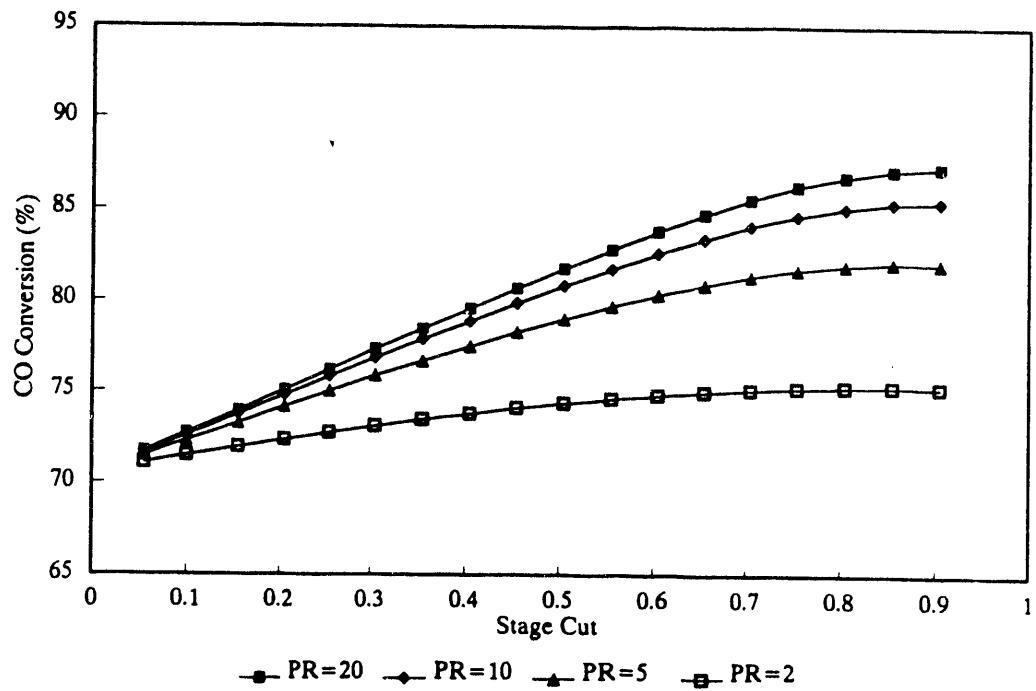
**Figure 5-3. Effect of stage cut and pressure ratio on CO conversion, MTCI gasifier gas composition,  $\text{H}_2\text{O}:\text{CO} = 3:1$ .**
