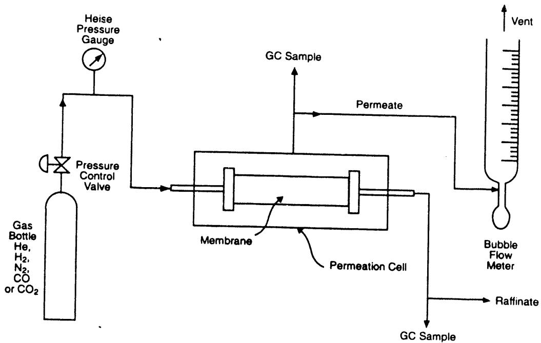
**Figure 3-2. Schematic of a permeation cell test apparatus.**
