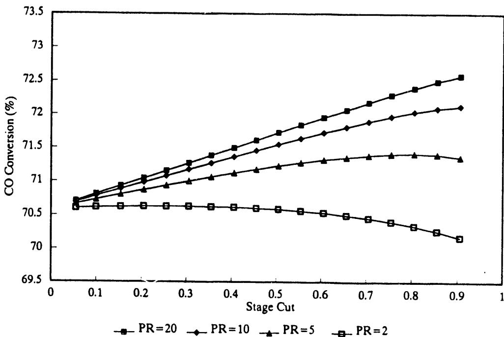
**Figure 5-8. Effect of stage cut and pressure ratio on CO conversion, low gas separation factors, MTCI gasifier gas composition,  $\text{H}_2\text{O}:\text{CO} = 3:1$ .**
