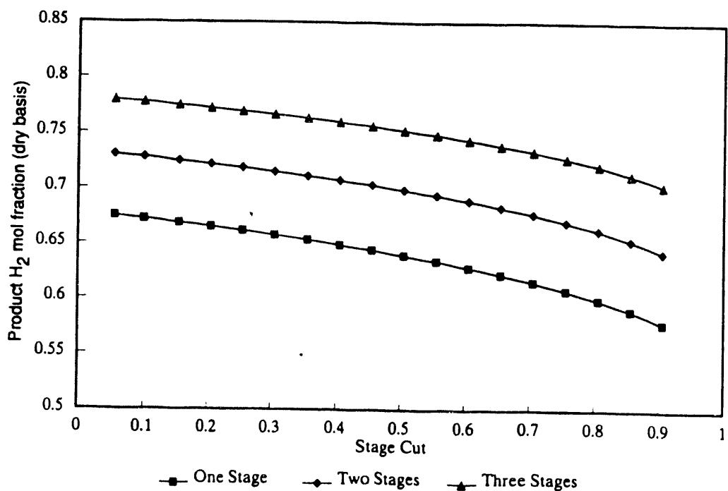
**Figure 5-11. Product  $H_2$  concentration with number of stages, MTCI gasifier gas composition,  $H_2O:CO = 3:1$ , low gas separation factors.**
