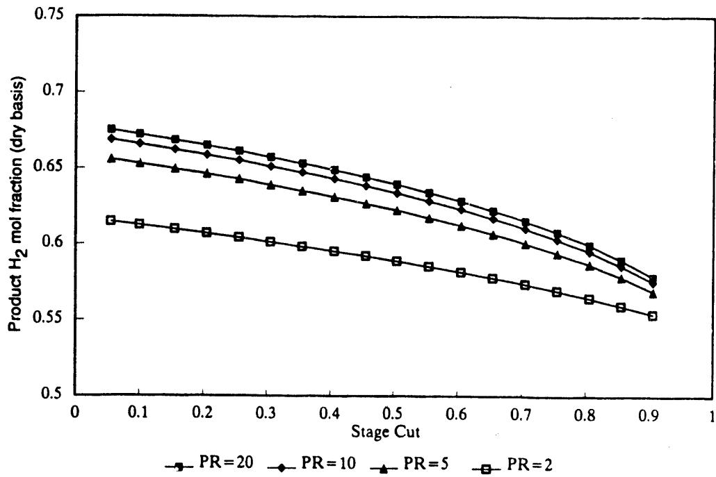
**Figure 5-9. Effect of stage cut and pressure ratio on product  $H_2$  concentration, low gas separation factors, MTCI gasifier gas composition,  $H_2O:CO = 3:1$ .**
