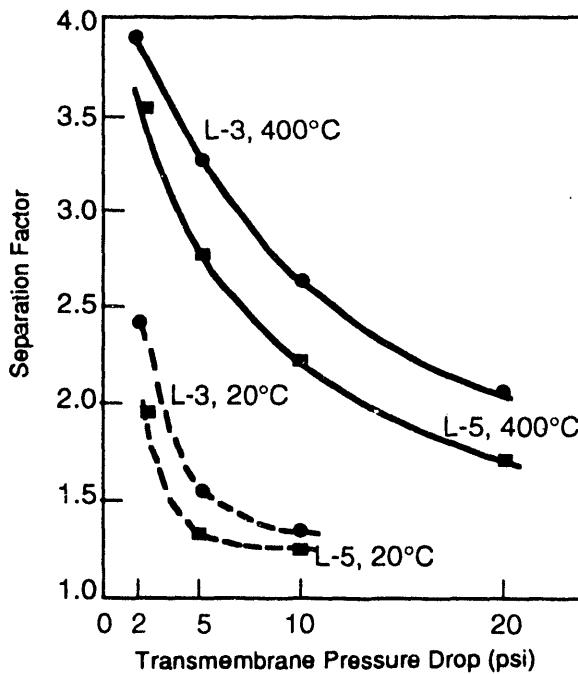
**Figure 4-4. Effect of temperature and transmembrane pressure drop on  $\text{H}_2/\text{CO}_2$  separation factor**
