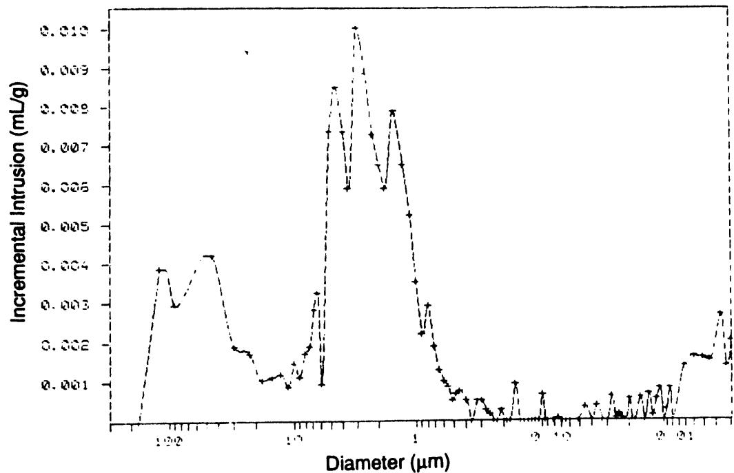
**Figure 3-4.** Pore size distribution for a 1.0- $\mu\text{m}$  unmodified carbon membrane sample.
