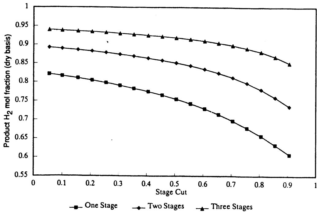
**Figure 5-10. Product  $H_2$  concentration with number of stages, MTCI gasifier gas composition,  $H_2O:CO = 3:1$ , Knudsen diffusion separation.**
