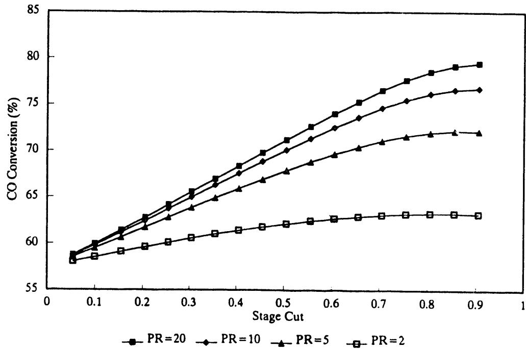
**Figure 5-2. Effect of stage cut and pressure ratio on CO conversion, MTCI gasifier gas composition,  $\text{H}_2\text{O}:\text{CO} = 2:1$ .**
