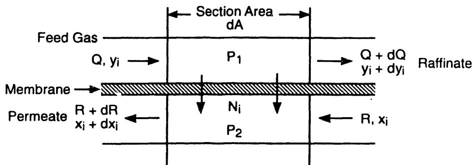
**Figure 5-1. Schematic of a membrane reactor system.**
