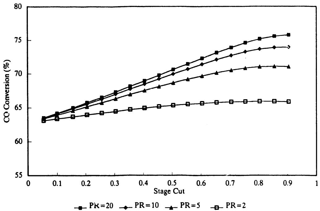
**Figure 5-12. Effect of stage cut and pressure ratio on CO conversion, Texaco gasifier gas composition,  $\text{H}_2\text{O}:\text{CO} = 1:1$ .**
