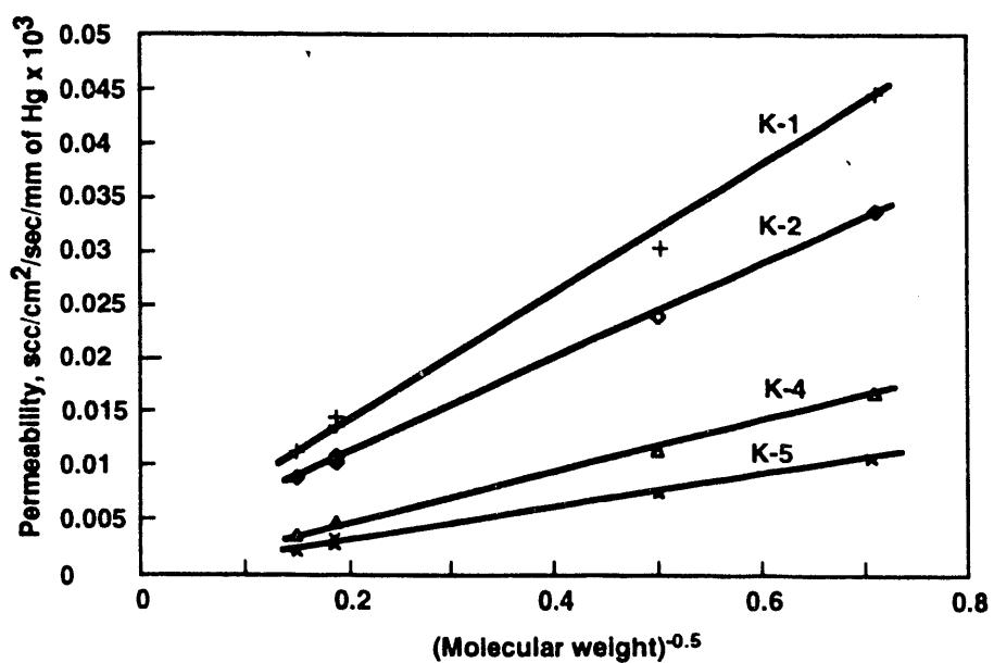
**Figure 3-8. Pure component permeabilities for various FAP resin-coated samples.**
