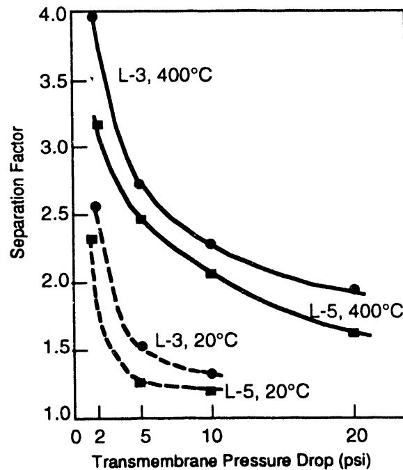
**Figure 4-3. Effect of temperature and transmembrane pressure drop on H<sub>2</sub>/CO separation factor.**
