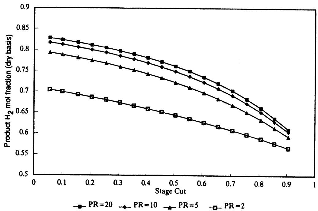
**Figure 5-14. Effect of stage cut and pressure ratio on product H<sub>2</sub> concentration, Texaco gasifier gas composition, H<sub>2</sub>O:CO = 2:1.**
