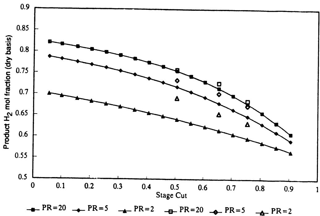
**Figure 5-7. Effect of flow scheme on product  $\text{H}_2$  concentration, MTCI gasifier gas composition,  $\text{H}_2\text{O}:\text{CO} = 3:1$ .**
