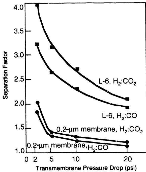
**Figure 4-2. Observed gas separation factors at 400 °C for an unmodified membrane and membrane sample L-6.**
