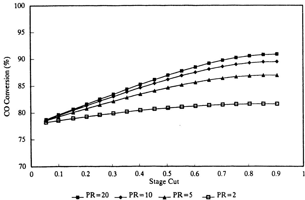
**Figure 5-4. Effect of stage cut and pressure ratio on CO conversion, MTCI gasifier gas composition,  $\text{H}_2\text{O:CO} = 4:1$ .**
