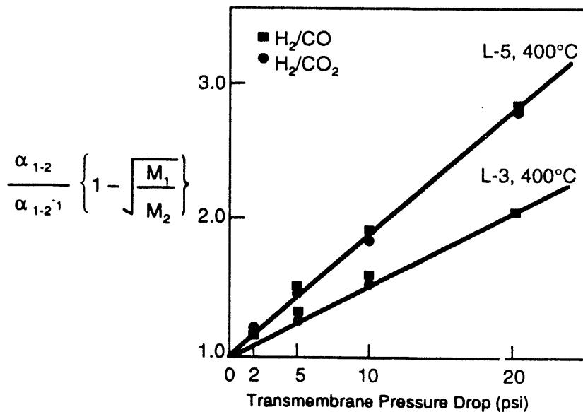
**Figure 4-5. Observed H<sub>2</sub>/CO and H<sub>2</sub>/CO<sub>2</sub> separation factor relationship with ΔP.**
