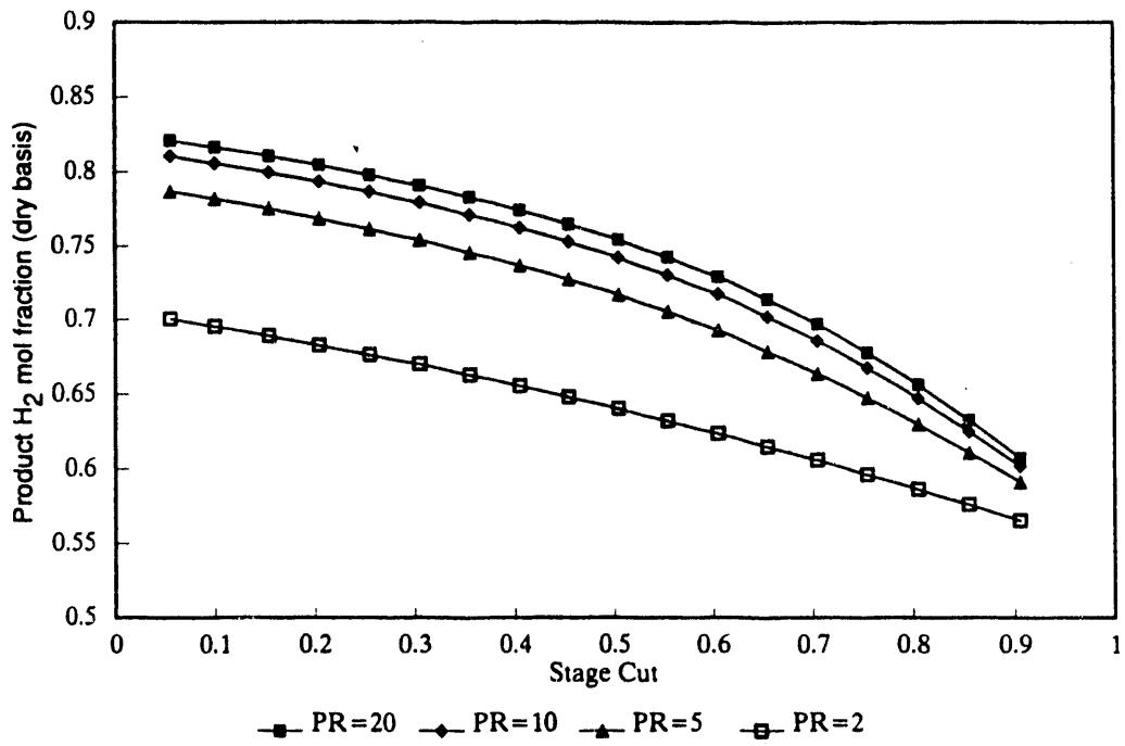
**Figure 5-5. Effect of stage cut and pressure ratio on product  $\text{H}_2$  concentration, MTCI gasifier gas composition,  $\text{H}_2\text{O:CO} = 3:1$ .**
