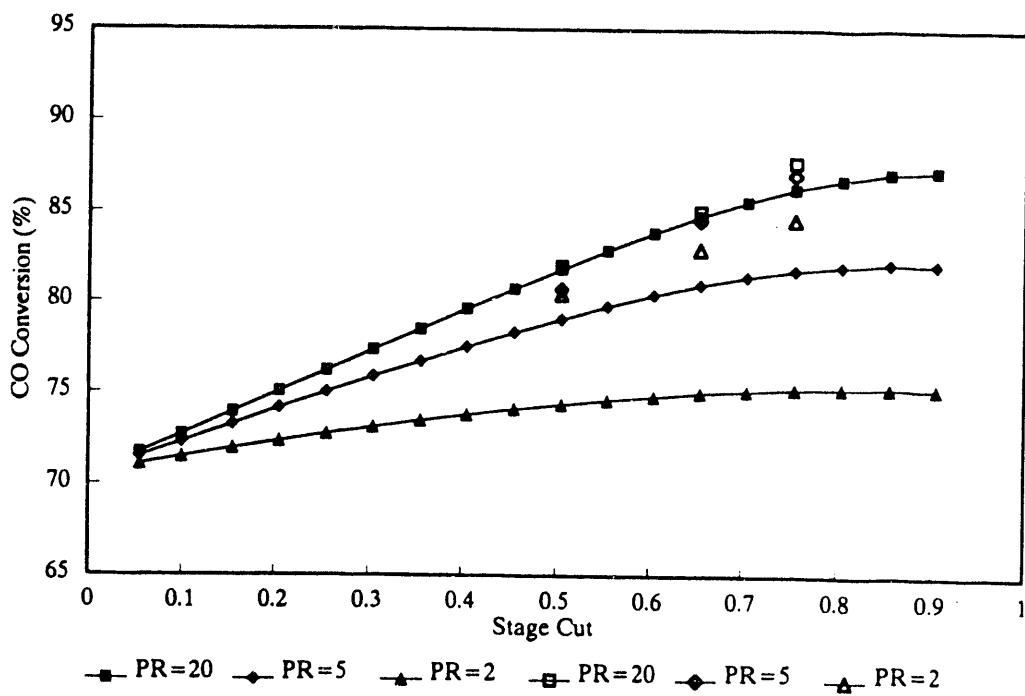
**Figure 5-6. Effect of flow scheme on CO conversion, MTCI gasifier gas composition,  $\text{H}_2\text{O}:\text{CO} = 3:1$ .**
