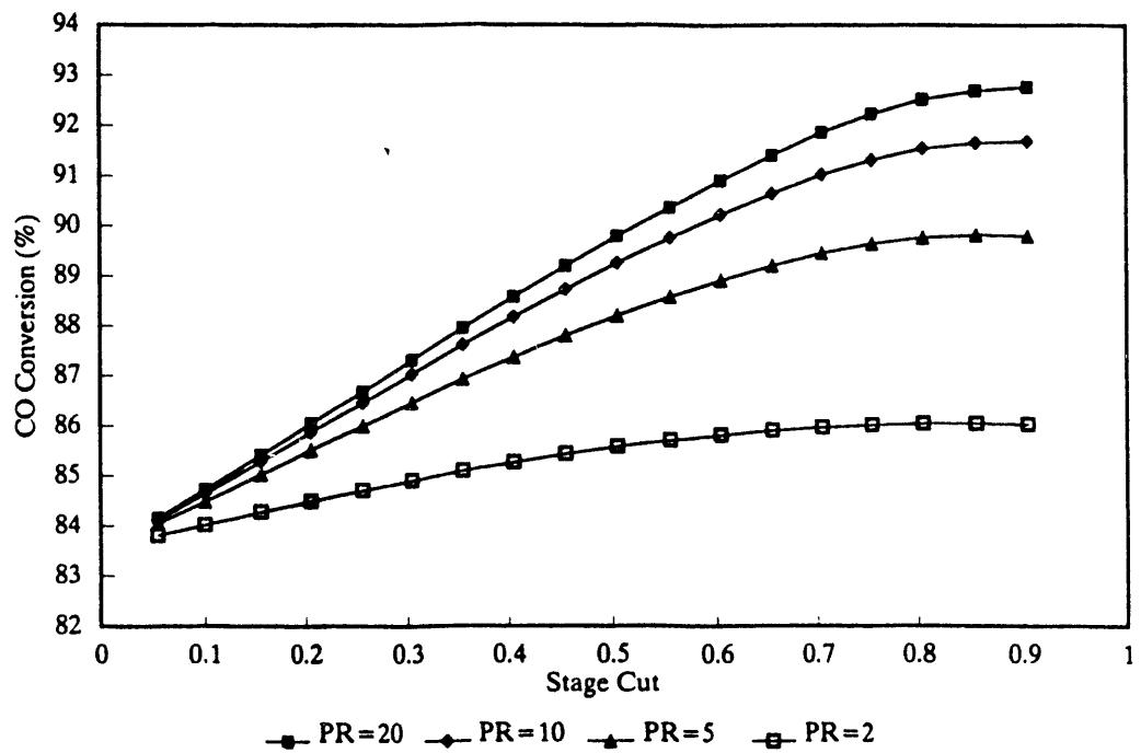
**Figure 5-13. Effect of stage cut and pressure ratio on CO conversion, Texaco gasifier gas composition,  $\text{H}_2\text{O}:\text{CO} = 2:1$ .**
