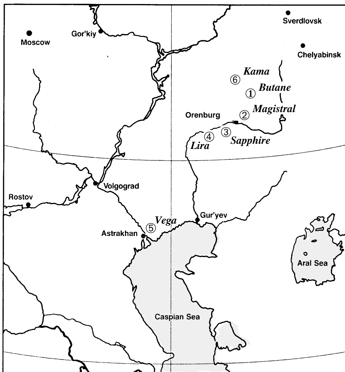
Figure 5. Map showing various PNE sites north of the Caspian Sea. (1) Butane is the first oil stimulation project. (2) Magistral, (3) Sapphire, (4) Lira, and (5) Vega are gas condensate storage projects. (6) Kama is the toxic waste storage project.
