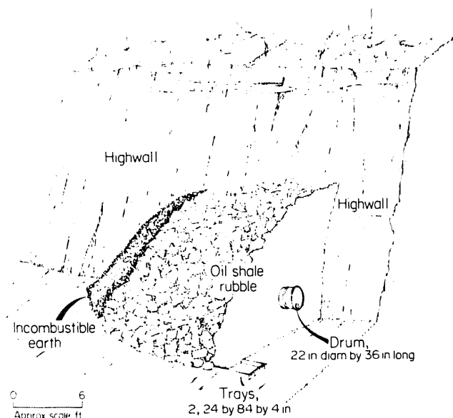
Figure 3-2.—Rubble pile configuration with heater.
