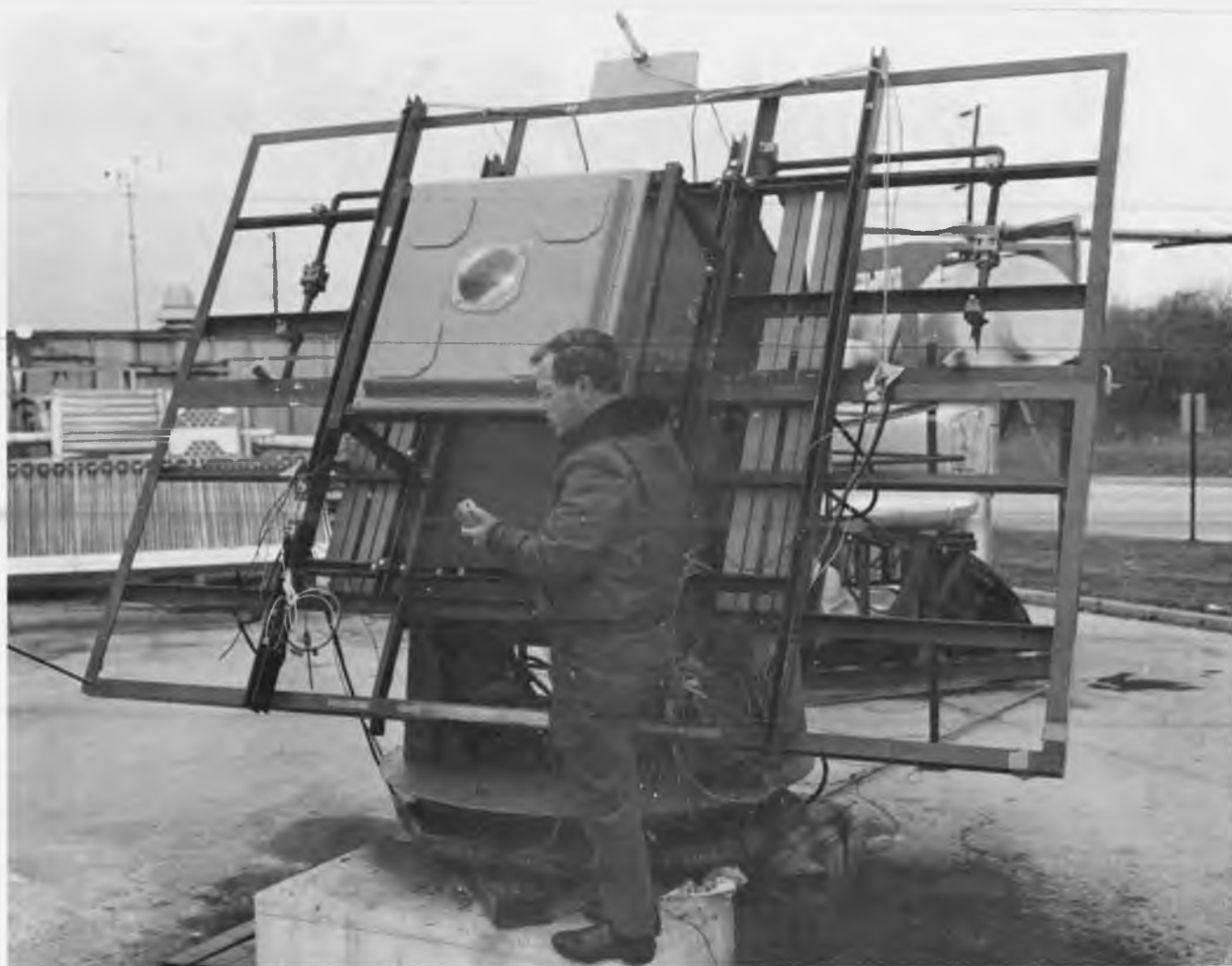
Figure 50. Prototype Module Mounted on Tracker Platform
