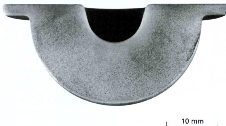
Figure 1. This micrograph shows a cross section of a thick-wall hemispherical forging produced by a two-stage process.
