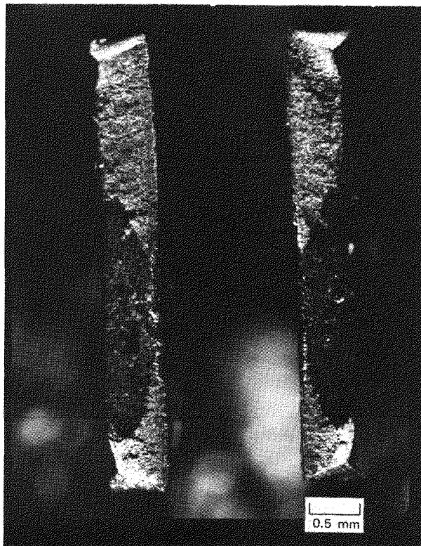
FIGURE 5-7 OPTICAL FRACTOGRAPH OF SPECIMEN Zr-4-18 SHOWING A WELL-DEFINED REGION OF SCC THAT PENETRATED ALMOST COMPLETELY THROUGH THE TUBING WALL
