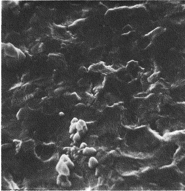
(a) AS RECEIVED, ANNEALED ZIRCALOY-2, 40-kg LOAD, 40 Pa I_2 , 30 MIN, 590 K, ION MILLED 60 MIN Width of photograph = 100 \mu m.
