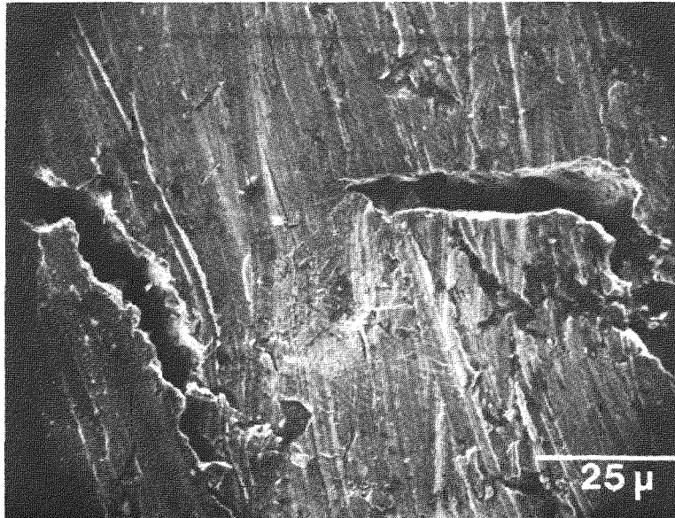
FIGURE 6-21 A PLASTICALLY DEFORMED BRIDGE IN A 4-POINT BEND SPECIMEN OF STRESS-RELIEVED ZIRCALOY-4 AFTER FAILURE IN THE ELASTIC REGION IN CADMIUM AT 633 K
