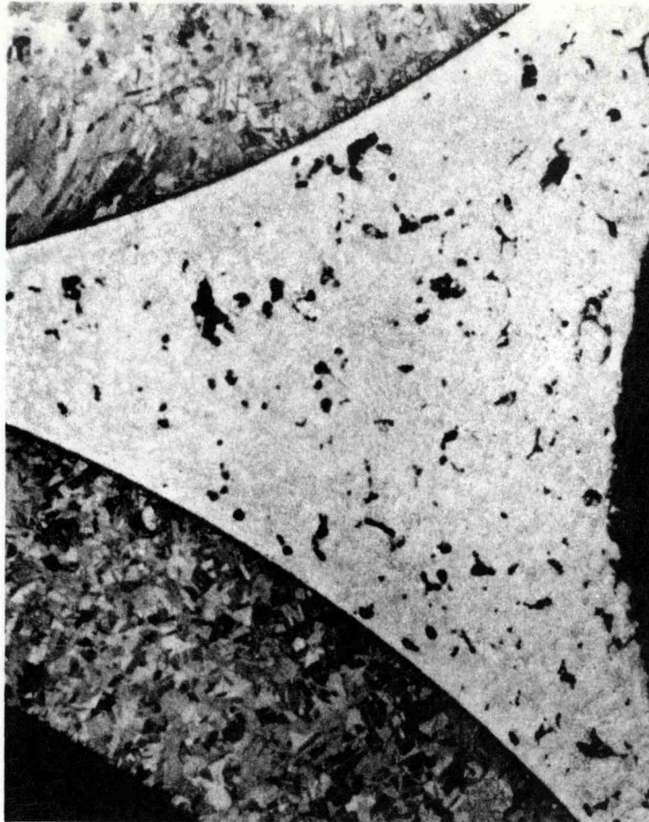
Figure 2-20. Results of Sintering the Non-Melting Powder NG108, Then Infiltrating with Brazing Filler Metal NB LM (30X Magnification)
