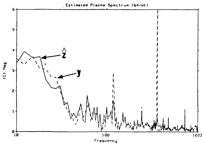
Figure 7 Real-Time Noise Canceller Design: (a) Plasma Pulse; and (b) Spectra
