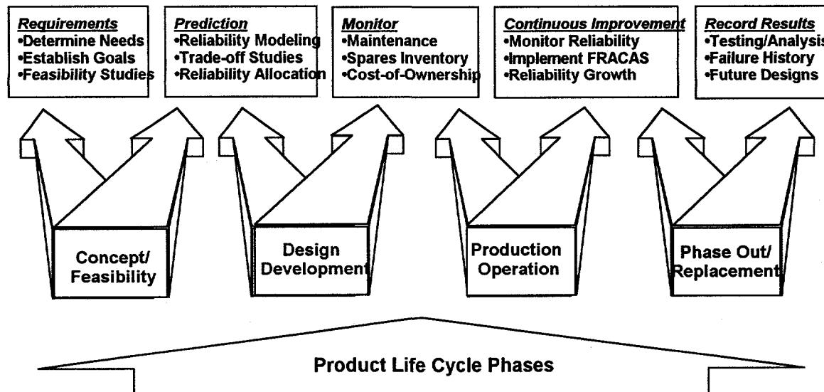
Figure 1. Typical phases and activities in the life cycle of a manufactured product.
