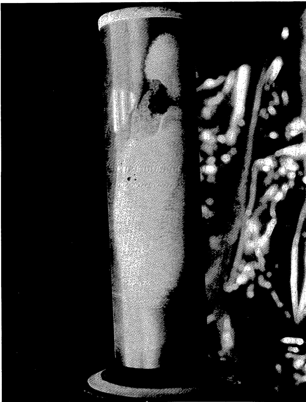
Fig. 18. View of Heat Pipe Defects Resulting from Hot Spot
