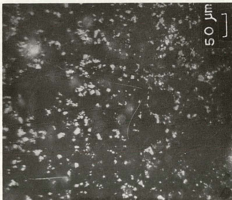
Figure C-24. PHOTOMICROGRAPH OF GLASSY SILICATE MATRIX WITH FERROUS ALUMINATE CRYSTALS IN COKE AGGLOMERATES
