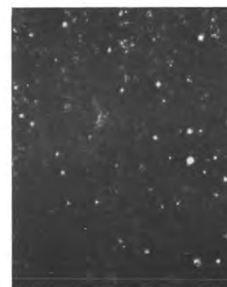
FIGURE 2. Darkfield Micrographs of Manufacture B Standard Mirrors Stressed for 336 Hours in 80°C Dry and Moist Environments
