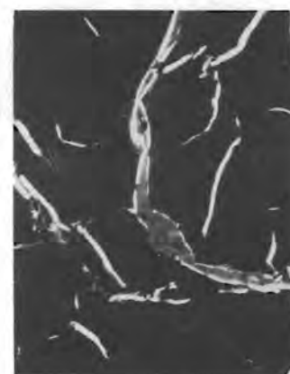
FIGURE 8. Darkfield Micrographs of the Ion Plated Silver, Nickel Backed Mirrors Stressed for 336 Hours at 80°C in Dry and Moist Environments
