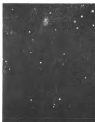
FIGURE 2. Darkfield Micrographs of Manufacture B Standard Mirrors Stressed for 336 Hours in 80°C Dry and Moist Environments
