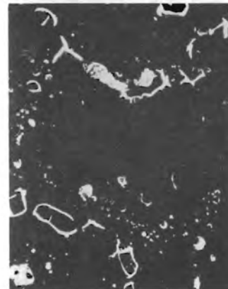
FIGURE 4. Darkfield Micrographs of the Ion Plated Silver, Aluminum Backed Mirrors Stressed for 336 Hours at 80°C in Dry and Moist Environments
