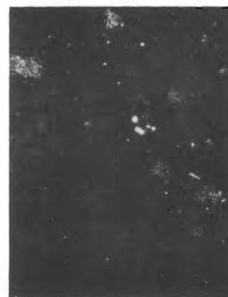
FIGURE 3. Darkfield Micrographs of Manufacture C Standard Mirrors Stressed for 336 Hours in the 80°C Dry and Moist Environments
