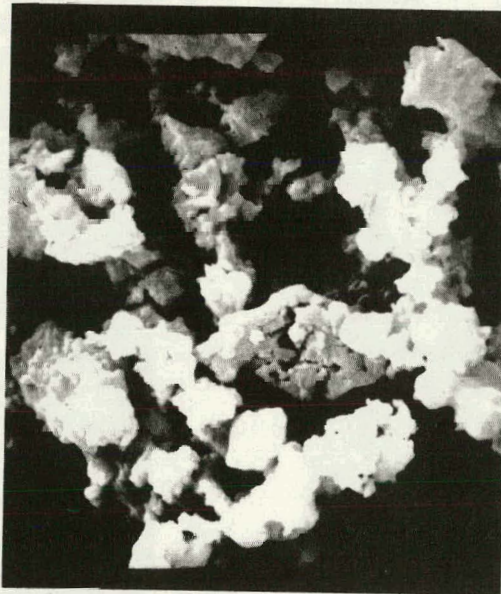
FIGURE 6-9. SEM photograph of -325-mesh calcined limestone particles after injection into flue gas at 2700°F.
