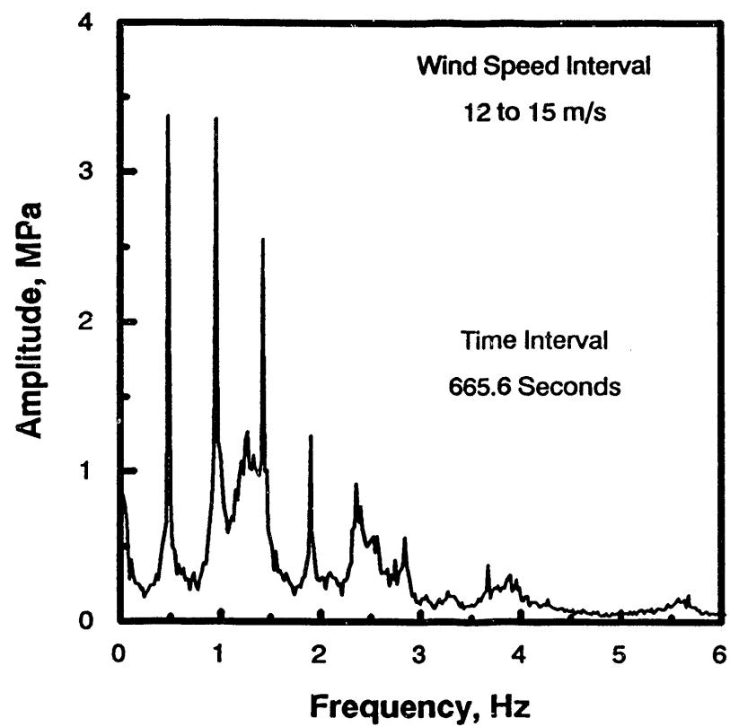
Figure 4. Average Amplitude Spectrum for the Sandia 34-m Test Bed with Small-Amplitude Phases Removed.
