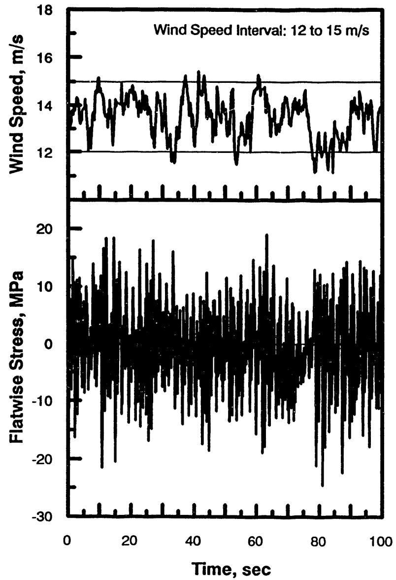
Figure 2. Single-Time-Series Amplitude Spectrum for the Sandia 34-m Test Bed.
