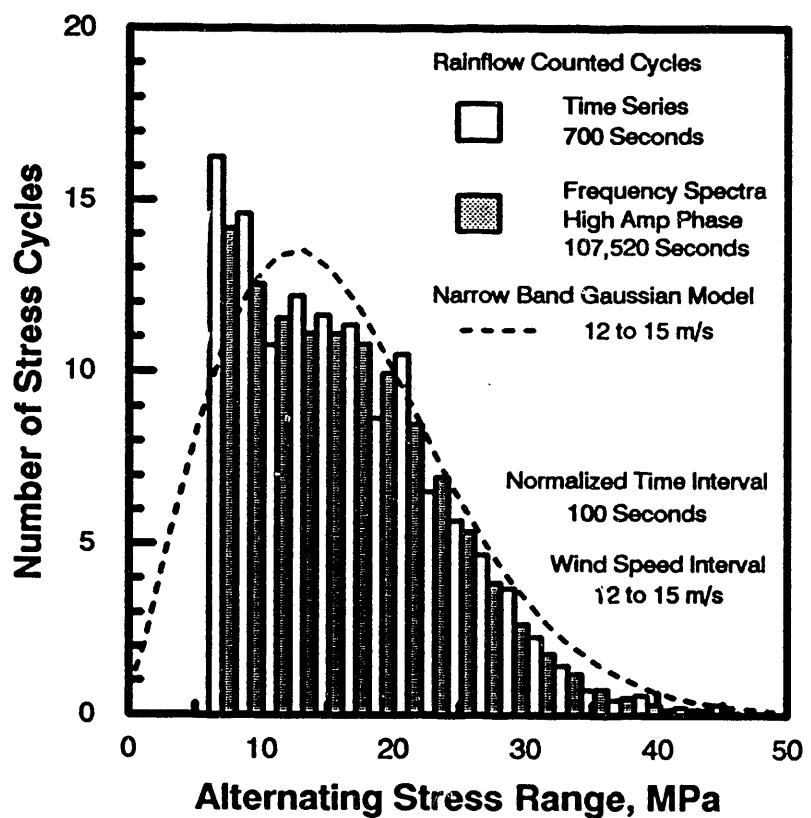
Figure 10. Cycle Counts for Time Series Synthesized with the RMS of the Input Frequency Spectrum Varying  $\pm 18$  Percent; Logarithmic Scale.
