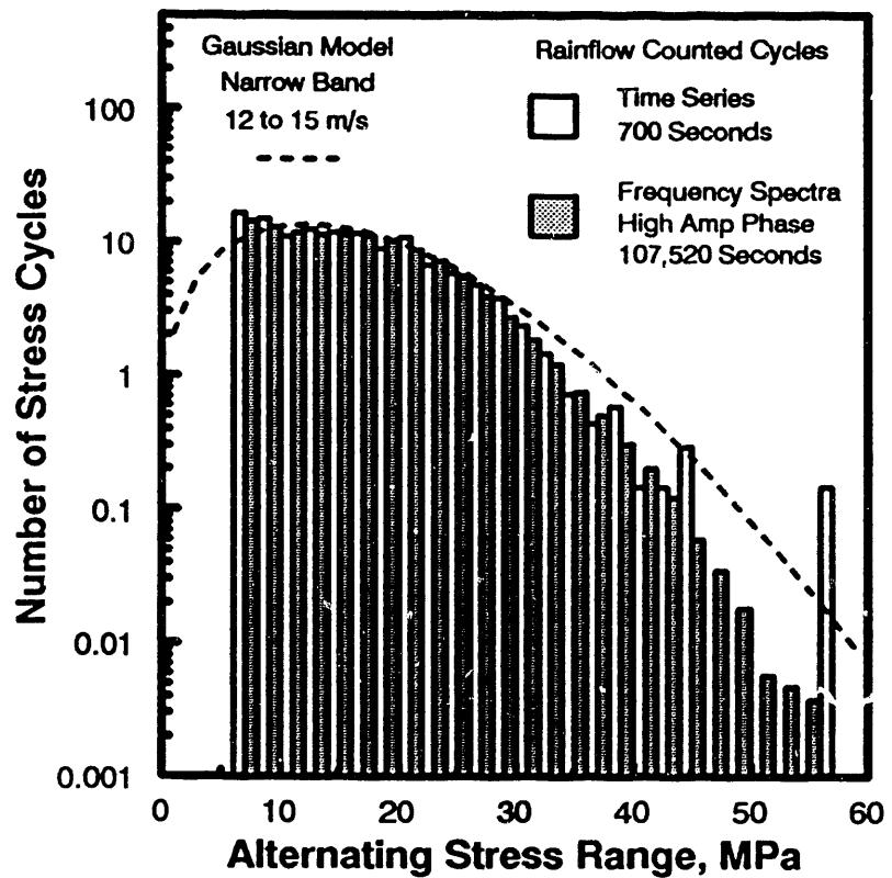
Figure 11. Cycle Counts for Time Series Synthesized with the Relative Small Amplitude Components Eliminated.
