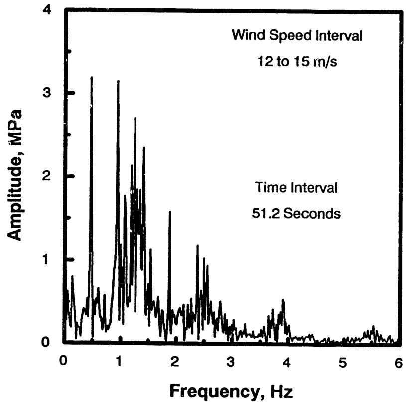
Figure 3. Average Amplitude Spectrum for the Sandia 34-m Test Bed.
