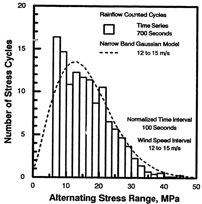
Figure 6. Cycle Counts for Time Series Synthesized from the Average Amplitude Spectrum with no Phase Angle.
