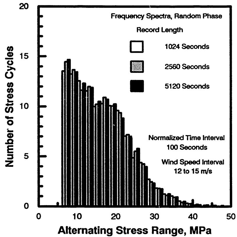
Figure 7. Cycle Counts for Time Series Synthesized from the Average Amplitude Spectrum with no Phase Angle.
