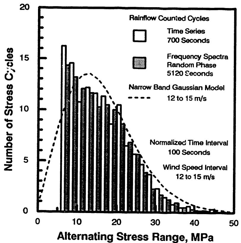
Figure 8. Cycle Counts for Time Series Synthesized from the Average Amplitude Spectrum with Phase Angles on the High-Amplitude Components.
