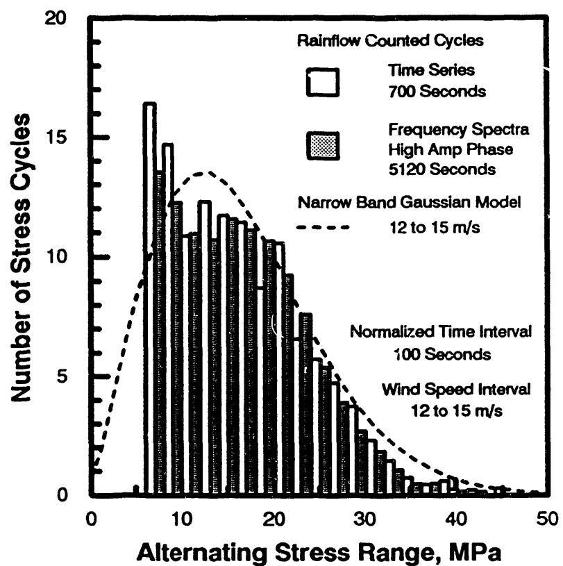
Figure 9. Cycle Counts for Time Series Synthesized with the RMS of the Input Frequency Spectrum Varying  $\pm 18$  Percent.
