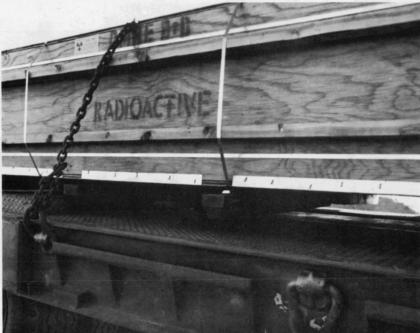
Figure 73. Soil box skids separating because support was inadequate.
