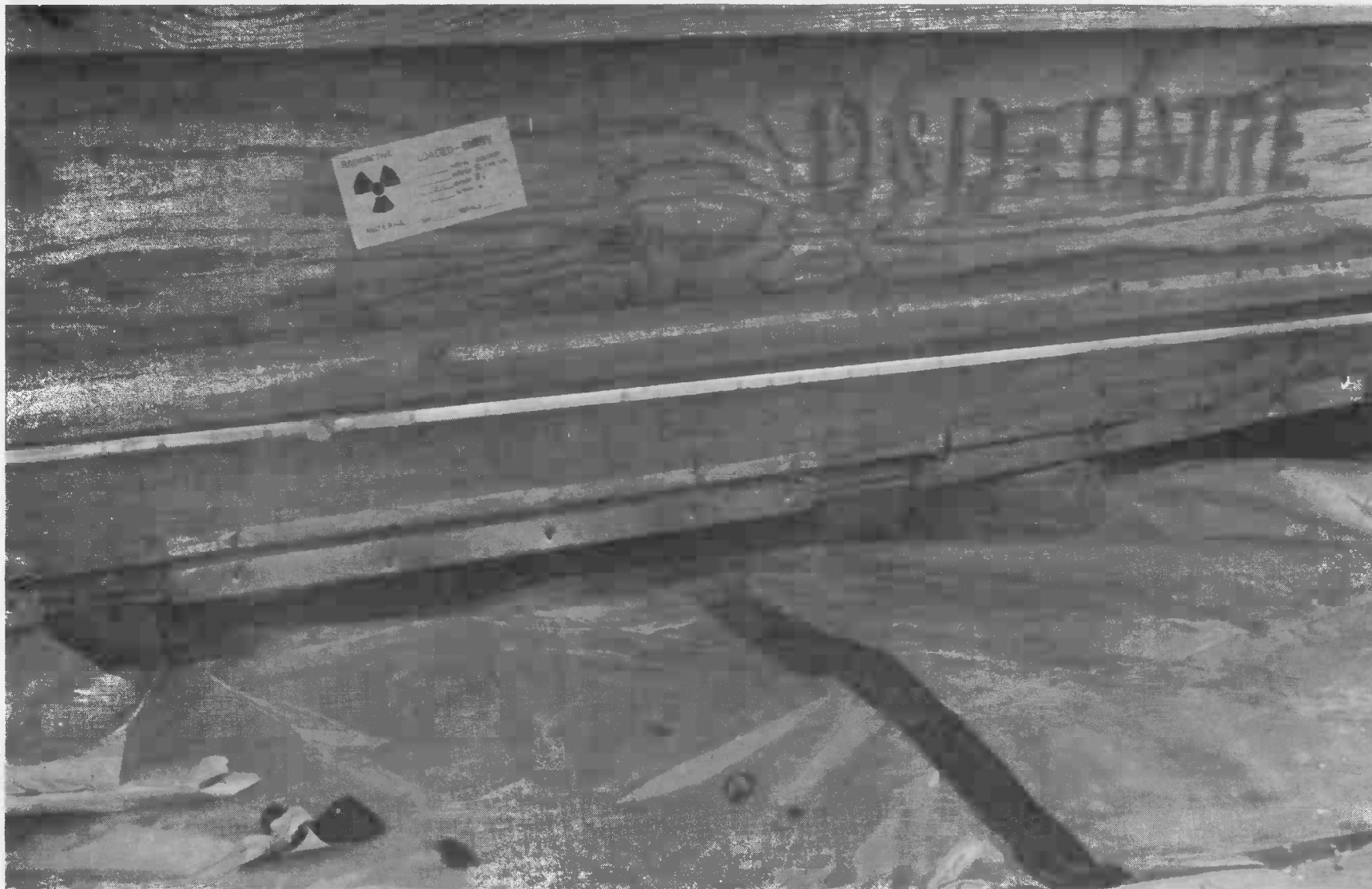
Figure 74. Ruptured bottom seam of soil box.
