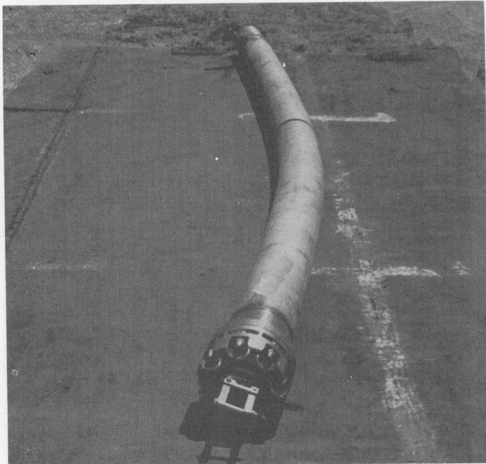
Figure 4-28 Canister After Two End-On Impact Tests
