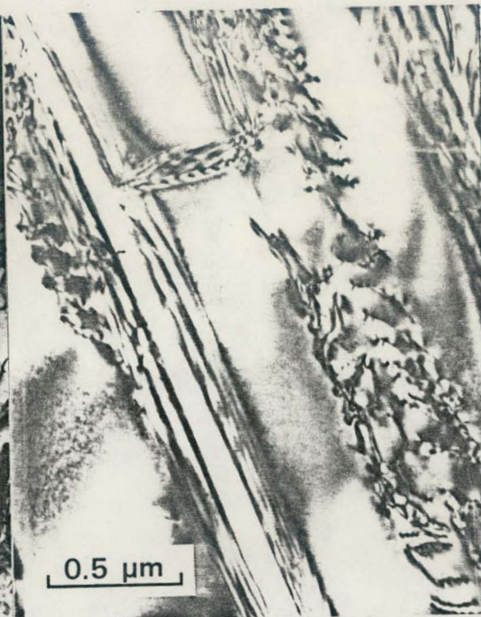
Figure 8. Part of Fig. 3, tilted to emphasize the contrast at a twin. Boundary fringes and interface dislocations are visible at the border of the twin.
