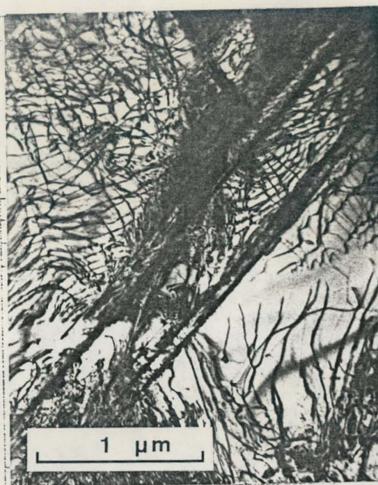
Figure 7. View of a basal plane nearly parallel to the photo plane. Note large networks and dislocation activity on planes normal to the basal plane.
