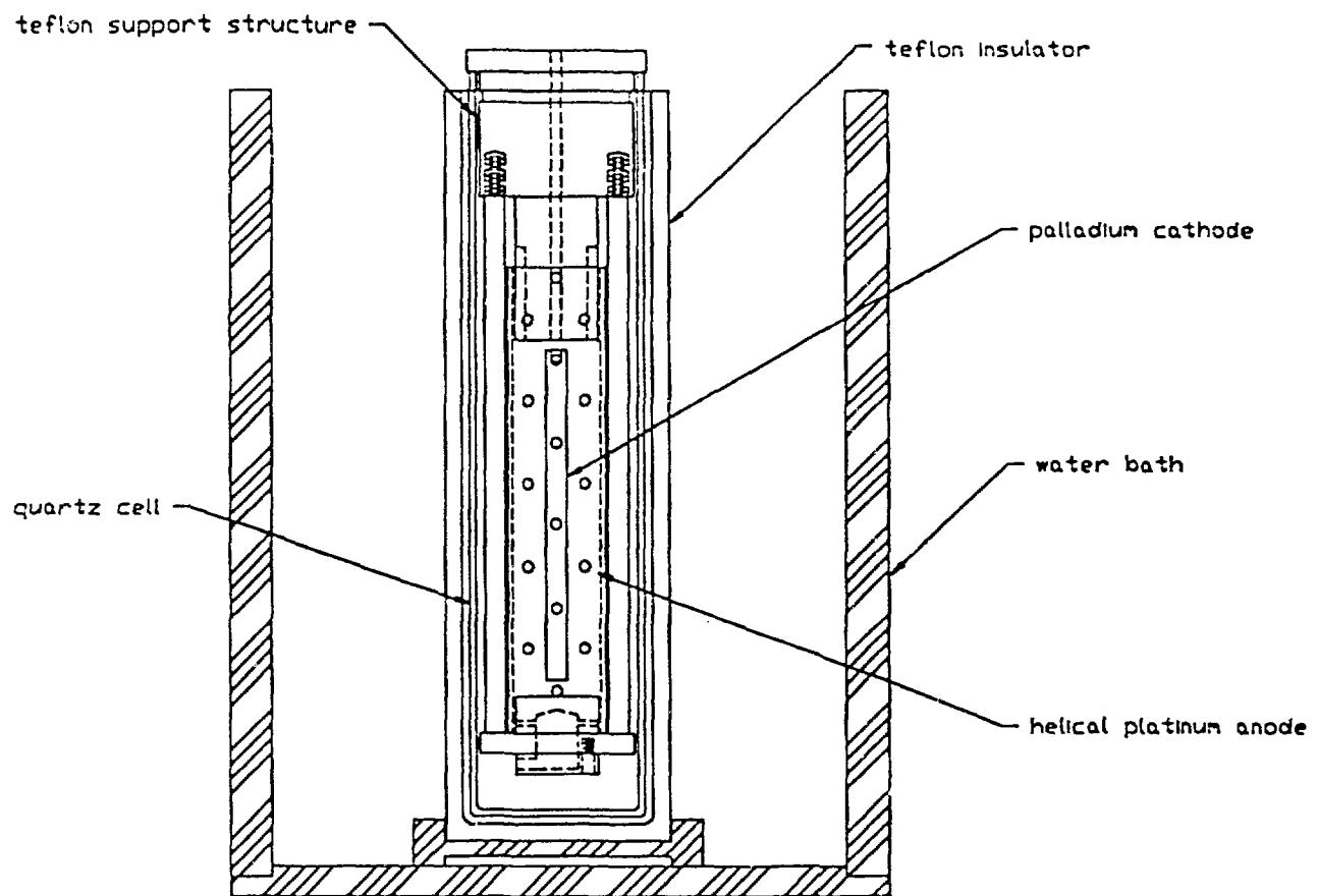
Fig. 1. Diagram of the design of the calorimetry cells.
