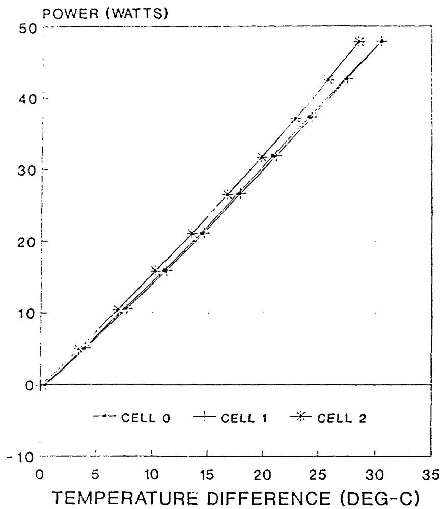
Fig. 2. Calibration curves for three of the calorimetry cells.
