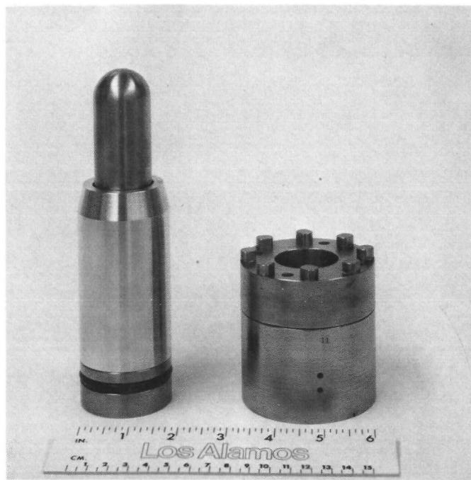
Fig. 3. Each test specimen was held in a two-piece molybdenum-alloy die (at right) and was impacted by a titanium-alloy punch (left).
