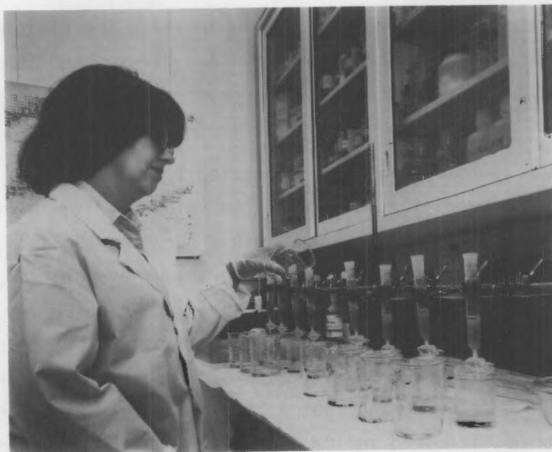
FIGURE 4. Separation of Uranium Using Ion Exchange Resins
