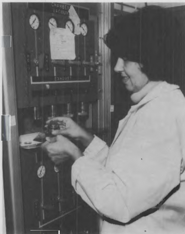
FIGURE 6. Measurement of Samples on Stainless Steel Discs Using a Multichannel Alpha Spectrometer
