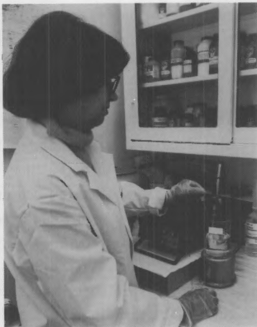
FIGURE 3. Co-Precipitation of Thorium on Ferric Hydroxide at Low pH
