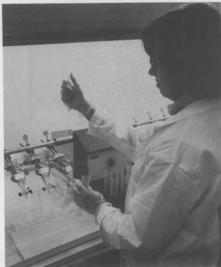
FIGURE 5. Thorium Fraction Purification by Extraction into Alamine-336 in Xylene
