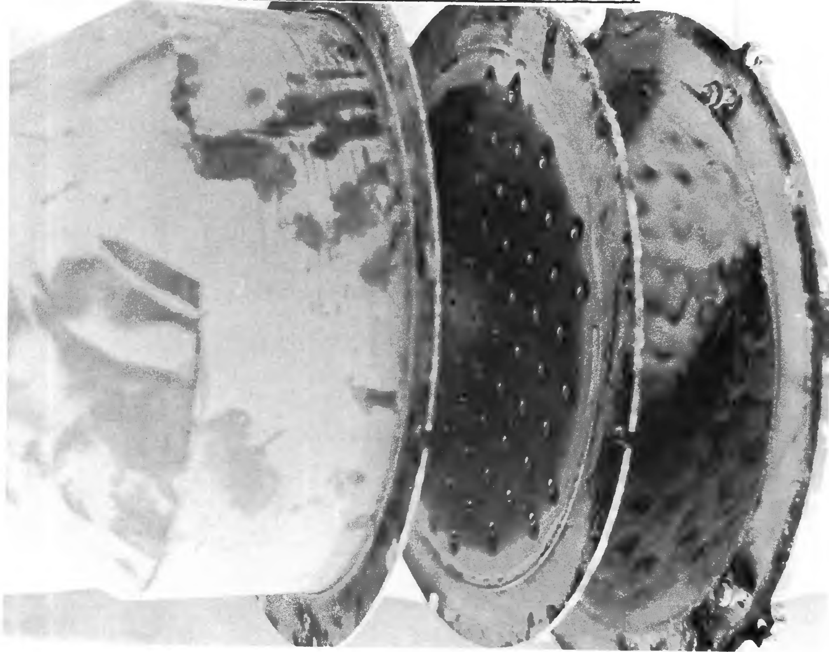
Turbine Test Section Flow Distributor Plate and Conical Inlet After Shakedown (Upstream Face)
