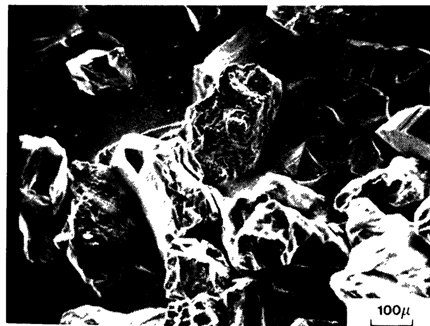
Fig. 3-1 - Scanning electron micrographs of the "washed" sand sample showing the smooth silicate surfaces and the uneven mixed oxide surfaces.
