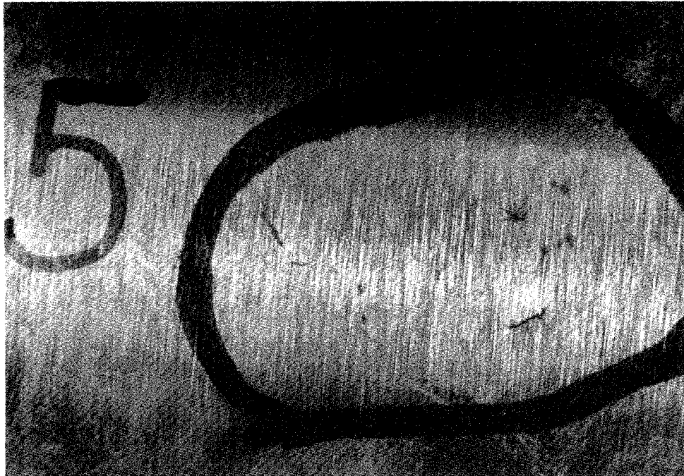
IMAGE 5 - 7X FLUORIDE CRACK. NOT FOUND BY EYE BUT PICKED UP USING DYE PENETRANT
