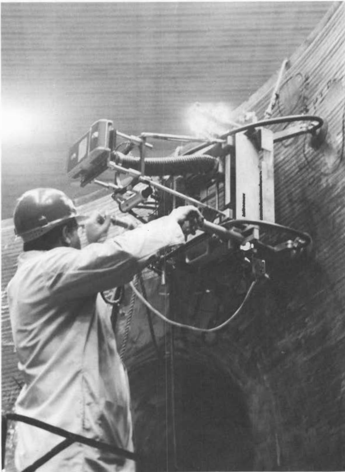
Figure 5-15 Operator Adjusting Scanner System During A Nozzle Weld Inspection (Mt. Vernon, Indiana)
