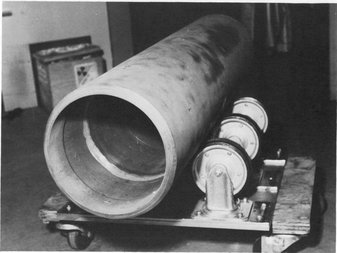
Fig. 6. Finished article of modified 9 Cr-1 Mo steel, which was sand blasted before final inspection. The weld root surfaces were ground smooth by hand.
