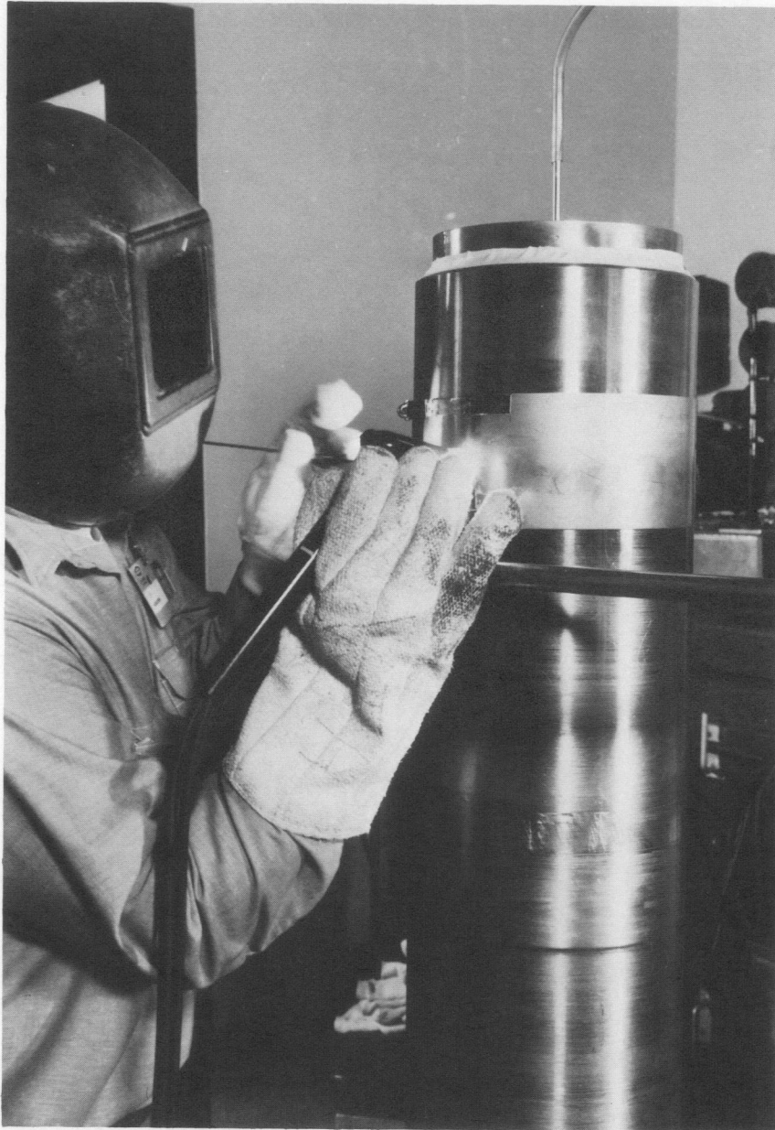
Fig. 5. Gas tungsten arc welding of modified 9 Cr-1 Mo steel test article in the 2G position.
