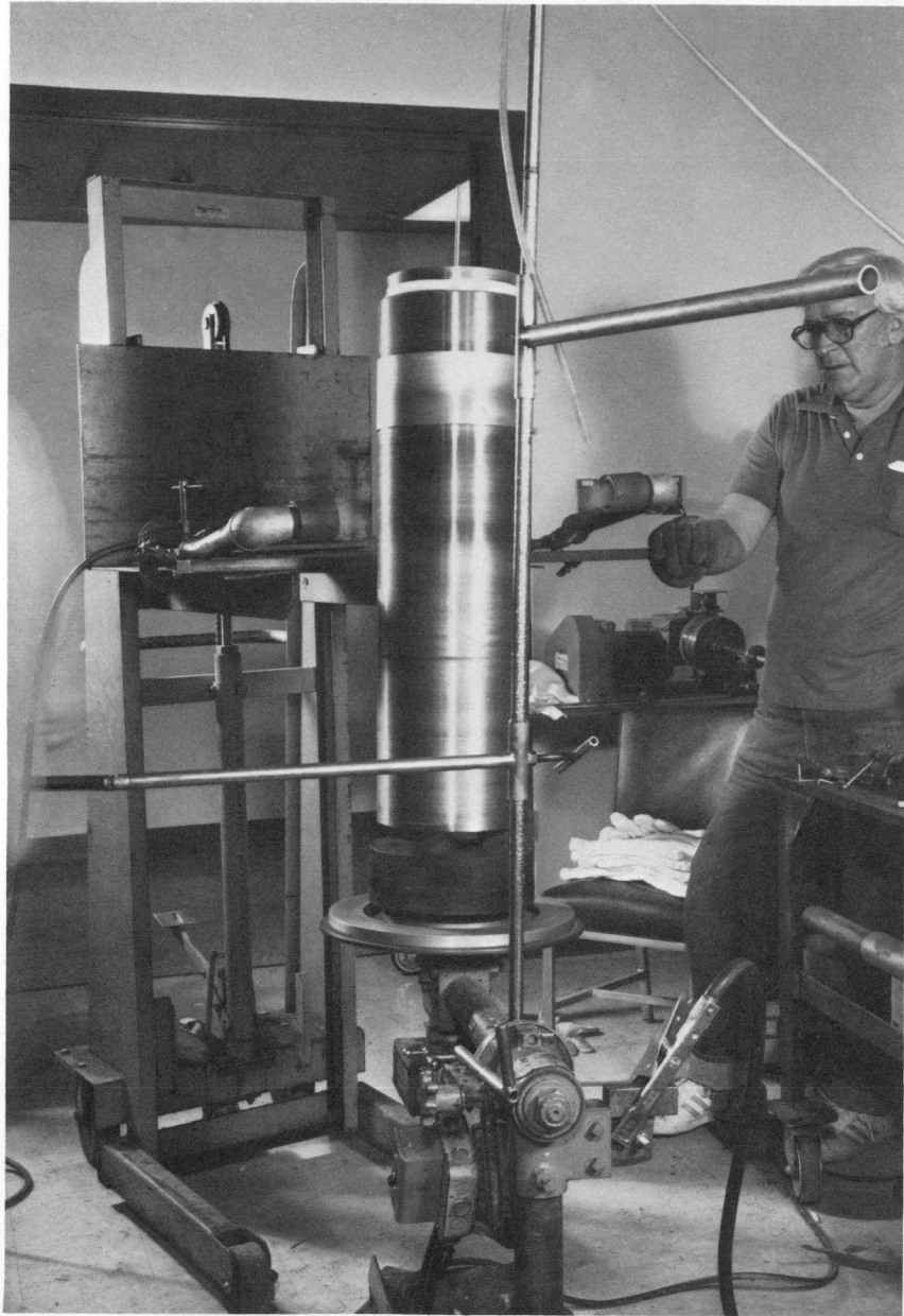
Fig. 4. Equipment setup for welding type 304L stainless steel end pieces to modified 9 Cr-1 Mo steel test article. Propane torches supply a preheat of 204°C minimum.
