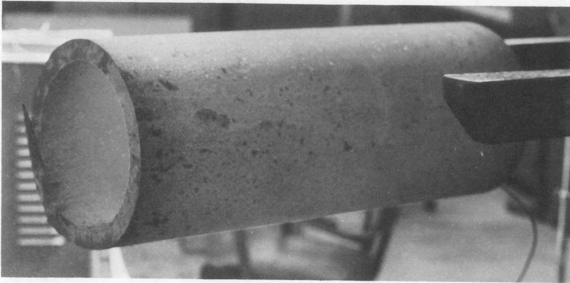
Fig. 1. Modified 9 Cr-1 Mo pipe air cooling from normalizing temperature of 1040°C to room temperature. The pipe dimensions were 245-mm OD by 25-mm wall by 610-mm length.
