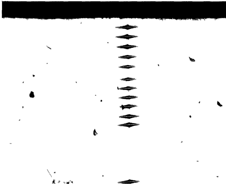
Figure 17. Knoop microhardness traverses in a sectioned Incoloy 800H high cycle fatigue specimen tested at 649°C (1200°F) in air; specimen MNF-164. Magnification 250X.
