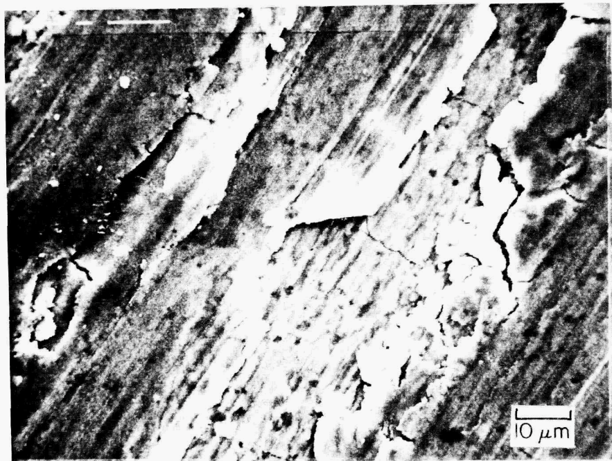
Figure 6. YPSZ wear surface lubricated with \text{MoS}_2 .
