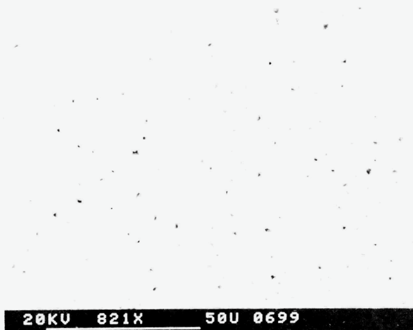
Fig. 7: 2.2 w/o \text{MgO-ZrO}_2 , made by melting baddeleyite and \text{MgO} , sintered at 1600^\circ\text{C} , polished and aged at 1400^\circ\text{C} for 1 hour.
