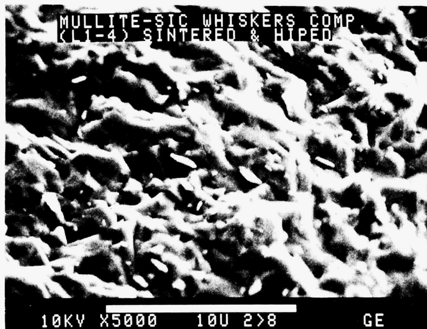
FIGURE 13 A FRACTURE SURFACE MULLITE-SiC (70/30, WT %) COMPOSITE NO. L1
