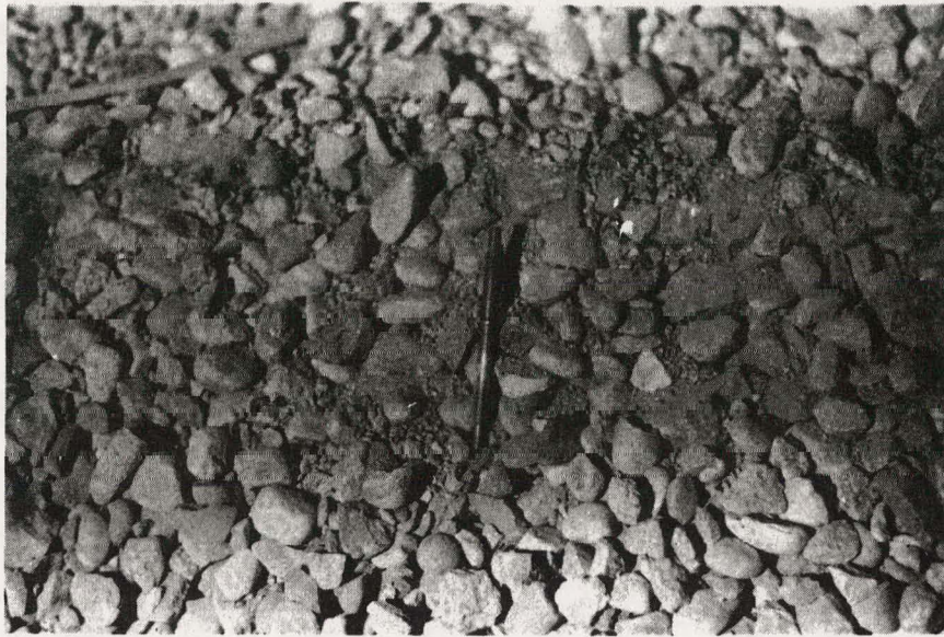
Figure 9-7. Fine Material within the Pebble Bed
