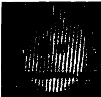
Fig. 71. A shear interferogram resulting from the reflection of a laser beam from a spherical mirror (10 m radius of curvature) with a 2 mm hole in the center.
