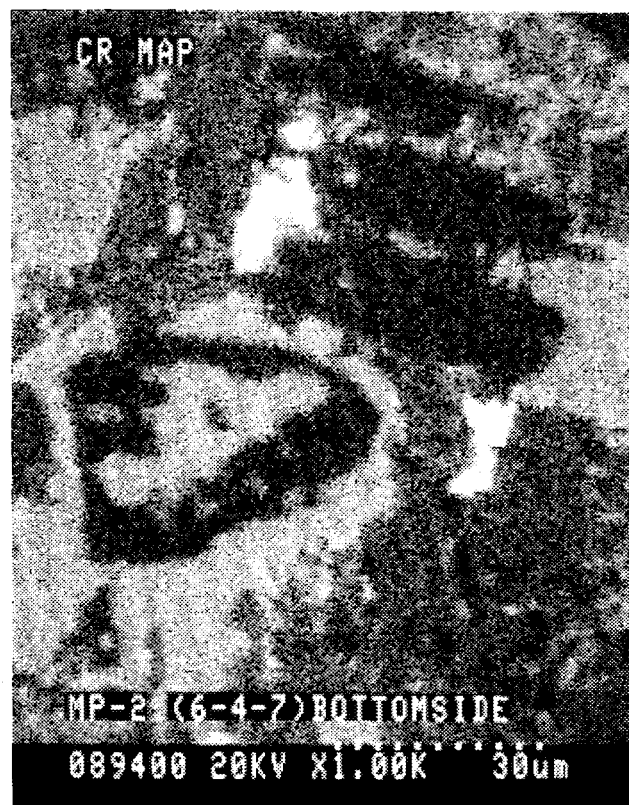
Figure C-2.7c Scanning Electron Micrographs and Corresponding Elemental Maps for the Relocated Material in the Bottom of the Test Capsule (RM-2.5)
