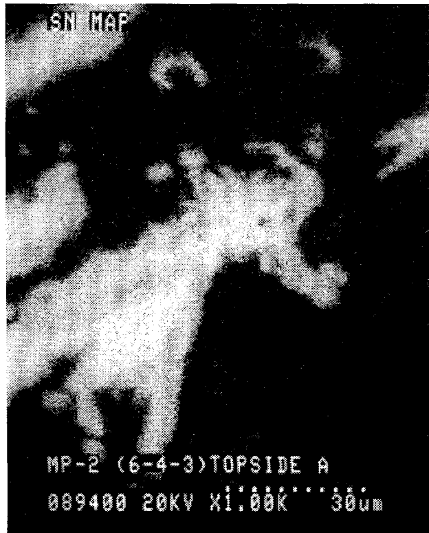
Figure C-2.6d Scanning Electron Micrographs and Corresponding Elemental Maps for the Relocated Material in the Mid-Section of Fuel Array (RM-2*)
