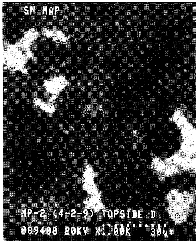
Figure 3.20d Scanning Electron Micrographs and Corresponding Elemental Maps for the Metallic Crust Remnant
