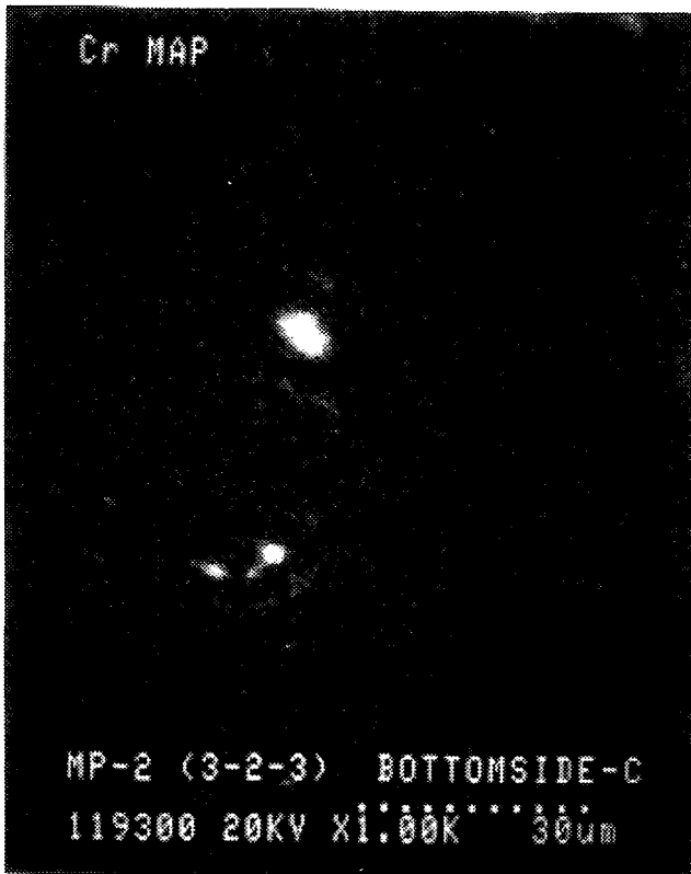
Figure 3.13d Scanning Electron Micrographs and Corresponding Elemental Maps for the Top of the Ceramic Melt Pool
