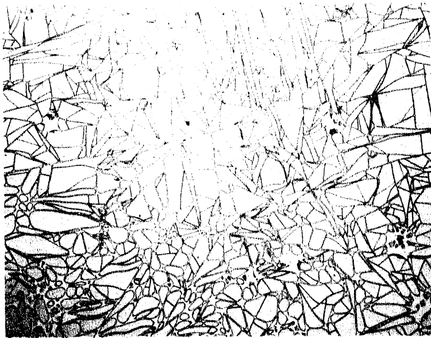
Figure 4.2a Optical micrograph of a fractured zirconia film on a quartz substrate.
