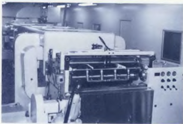
Figure 2. 3,000cm 2 class electrolyte plate manufacturing apparatus
