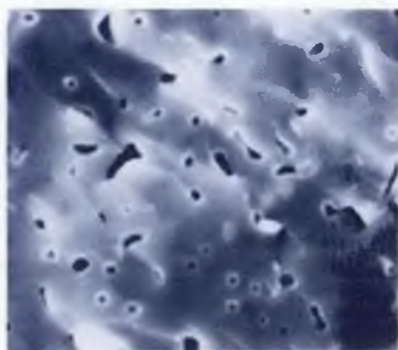
Fig. 4 Fracture surface (left) of 94% dense tape cast YSZ, and thermally etched surface (right) of 97% dense tape cast YSZ.
