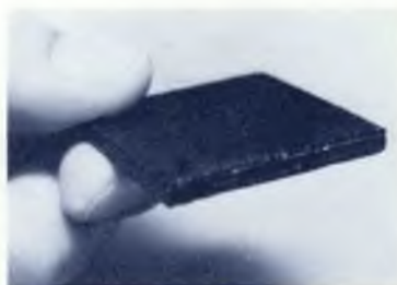
Figure 2. Sintered four-cell stack. Flat, well bonded structure free from visible cracks.
