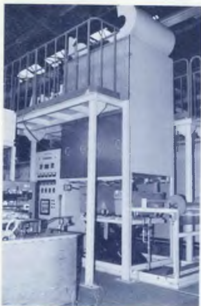
Figure 1. 3,000cm 2 class electrode manufacturing apparatus
