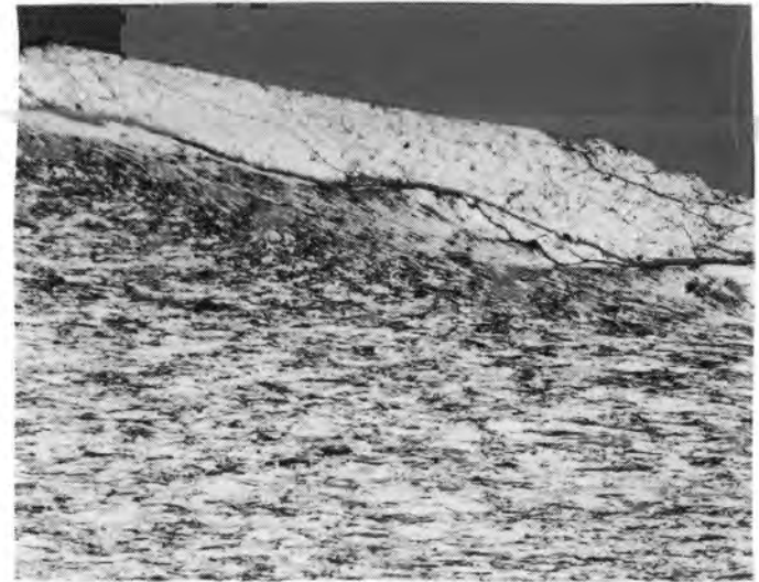
a. Wear Between IWRC and Strand Wire
