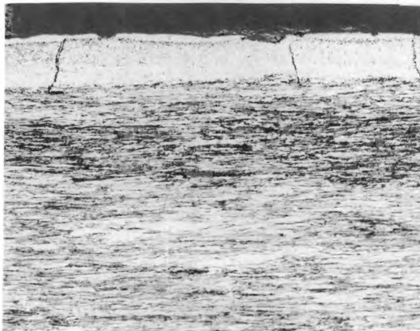
FIGURE 5.2. Martensite Formation on Field Rope Wire
