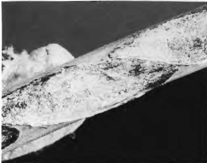
FIGURE 5.3. Photomicrographs of Wear on Field Rope
