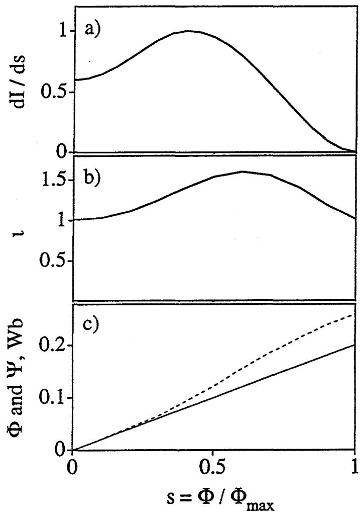
Fig. 4. Radial profiles in SSP of (a) normalized toroidal current density, (b) rotational transform, (c) toroidal (solid line) and poloidal (dashed line) magnetic fluxes.
