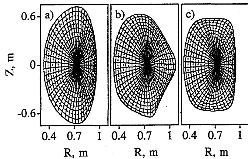
Fig. 3. High- $\beta$  equilibrium in SSP; a)  $\varphi = 0$ , b)  $\varphi = \pi/(2N)$ , c)  $\varphi = \pi/N$ .
