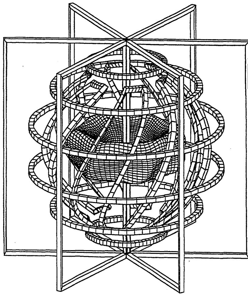
Fig. 1. Side view of the device considered and the last closed vacuum flux surface. The corresponding SSP is obtained by removing the rectangular TF coils.
